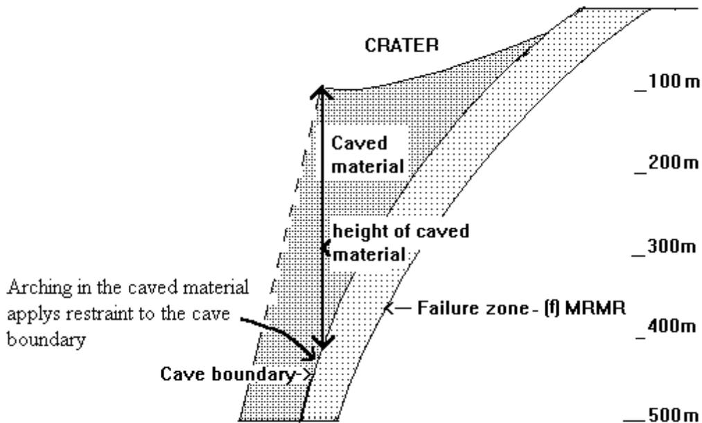
The failure zone is function of the MRMR. Ratings and zone widths are :-
