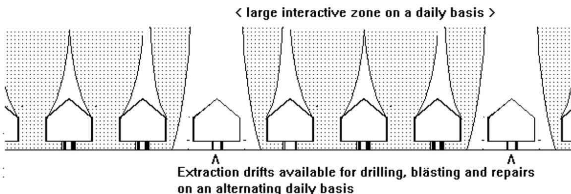
In fig 2 alternate production drifts are drawn. If there is uniform draw, and the production drifts are drawn on alternate shifts as at Henderson Mine then in one day complete lines of drawbells will be drawn and the optimum interaction is obtained. At Henderson mine the closed production drift is used for repairs or if not, it is not ventilated, thereby saving in costs.
