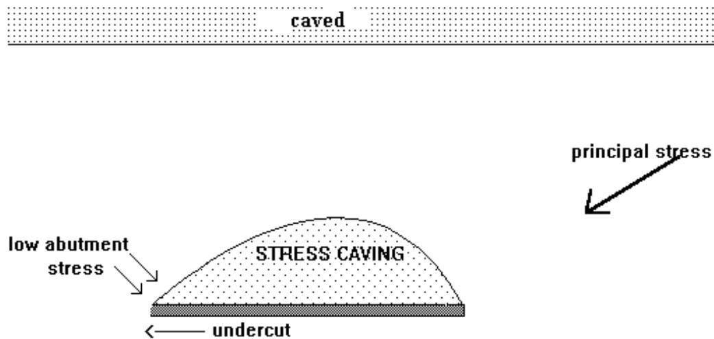
**Undercut away from principal stress = low abutment stress and poorer fragmentation**
