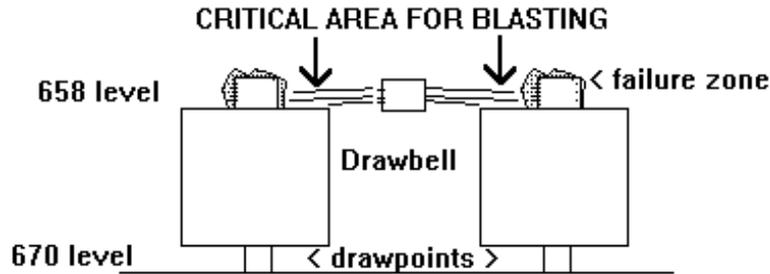
**Because the advance of the undercut is done ring by ring it is possible to check that the undercut is through before taking the next blast.** This is the procedure that was adopted in undercutting grizzly operations - the undercut would not be advanced until the operator was certain a connection had been made. In the large blasts of the conventional system it is assumed that the connection has been made - in many cases this is not the case.
