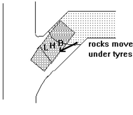
Techniques such as using the LHD bucket to break rocks on the floor of the drawpoint is not a good idea as the floor and LHD can be damaged leading to high maintenance costs.
