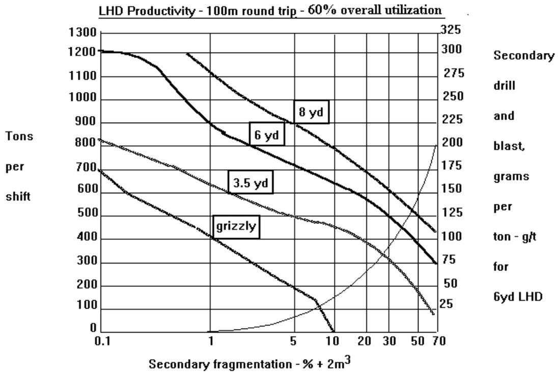
The range in fragmentation for different draw heights must be recorded as the average % + 2m<sup>3</sup> and should also reflect the range in particle size. This data will ensure that the productivity for the life of the block can be assessed. The LHD fleet could be reduced in time.
