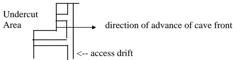
Advancing an undercut towards the principle stress should be avoided as this will result in high abutment stresses unless these stresses are necessary to induce caving and to improve the primary fragmentation:
