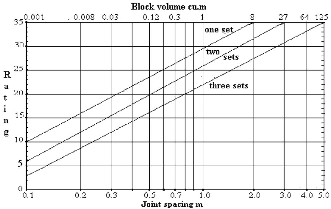
Figure 6. Joint spacing ratings
