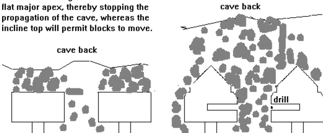
The incline advance undercut shapes the major apex from the undercut level.as shown in the following diagram
