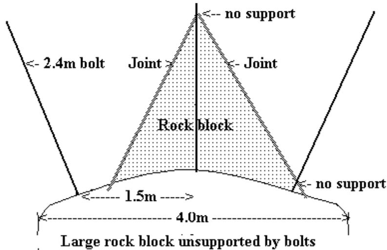
The following bolt pattern is suitable for most situations, the V in the back is preferred to the vertical bolt on the centre line:-
