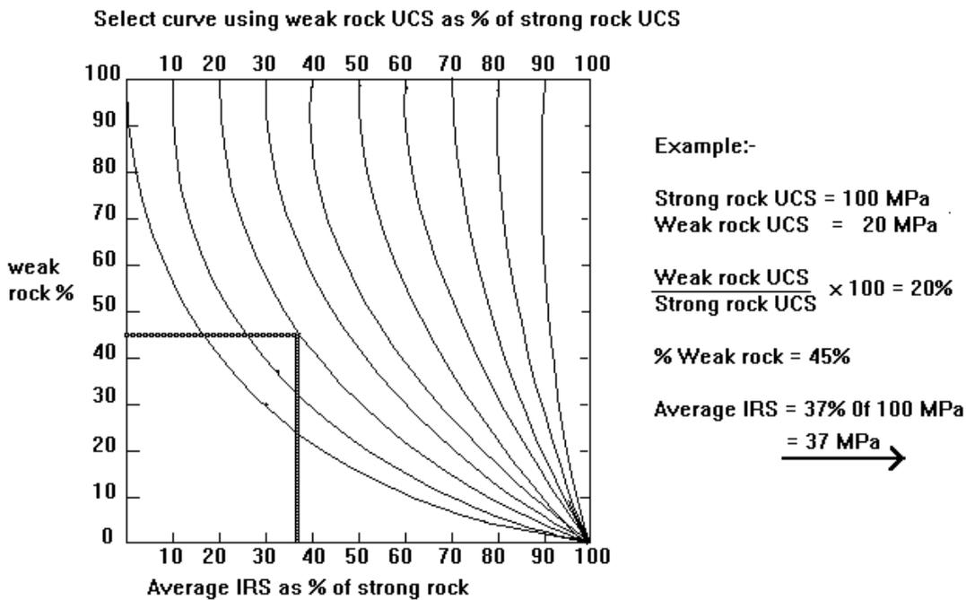
Figure 3. Nomogram for determining the “corrected” IRS value
