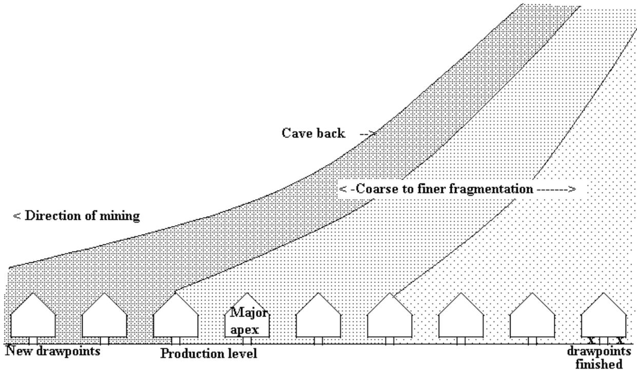
To achieve the same result with the caving of individual blocks, requires at least three blocks in operation simultaneously, but at different stages of draw. This requires excellent scheduling and can result in draw rates that are too low.
