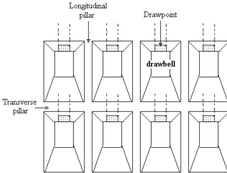
PLAN VIEW OF INCLINED EGGBOX LAYOUT
