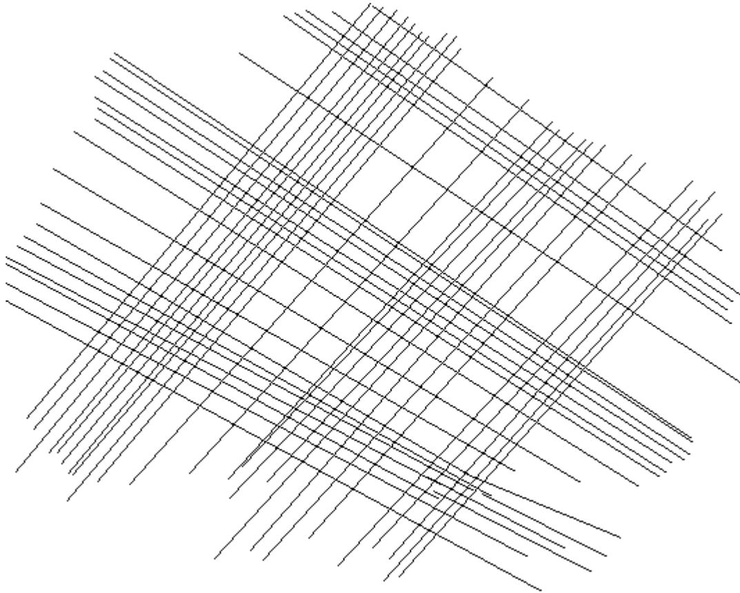
**Joint Condition Ratings** - Joint condition ratings must be assigned to individual joint sets as a set might have lower ratings than the others and therefore would always tend to fail before the others and would form a primary block boundary, whereas with the others it might only be every 2nd or 3rd joint e.g.:-
