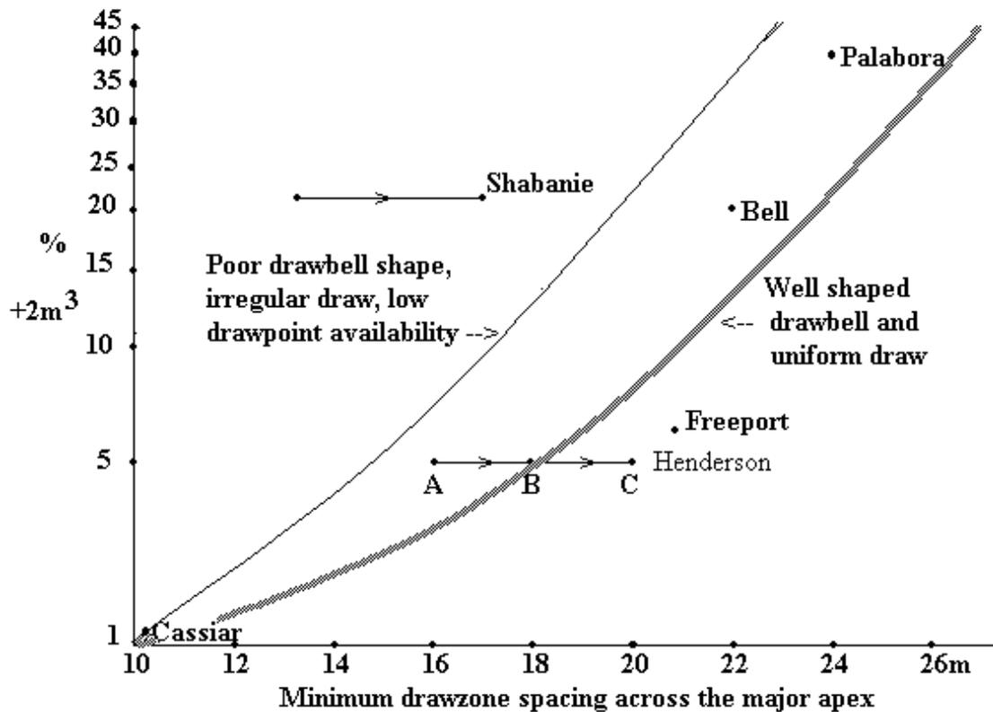
In the case of Henderson Mine, the spacing has been increased significantly. The question is how is PFC going to determine the spacing at Henderson? Examples of modelling predicting the answers to dynamic situations are required.
