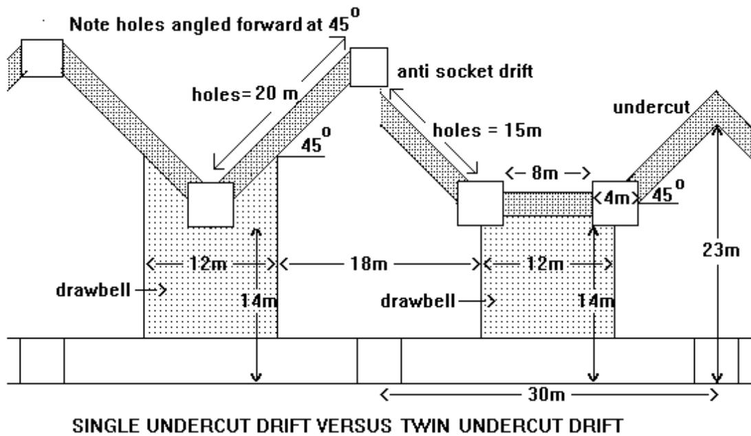
The advantage of the single drift layout is the assurance that the undercut has broken to the top of the major apex. Another advantage of the single undercut drilling drift is the reduction of development on a level, particularly at the access junction and this will minimise abutment stress damage. The major apex
