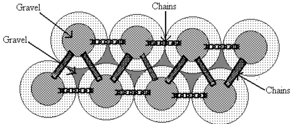
**Tyres joined with chains and filled with gravel on weak floors**
