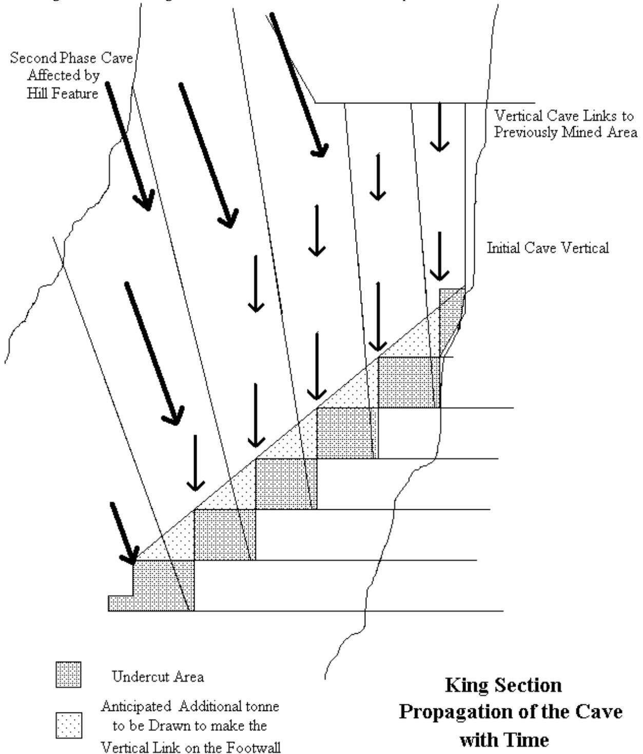
The caving of King Section Main Ore Body is believed to take place in phases. The initial cave being under gravity and the horizontal stresses, this cave progressing up the footwall side until it links to the previously caved block above. At this point once the strike has been opened far enough, a cave propagates through to surface on an incline and creates a loading of broken rock that 'pushes' the ore into an incline draw.
