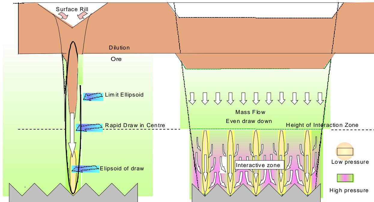
**Figure 2** Granular flow mechanisms – Material flow paths for drawpoints worked in isolation (left) and worked concurrently (right) where higher pressures in inter-drawpoint areas forces material into the low- pressure zones above working drawpoints.
