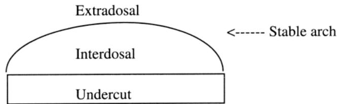
The interdossal zone contains caved material, the arch will only fail if the area is increased or boundary weakening is used either by slotting or blasting of the arch legs. The danger with boundary weakening is that a stable arch can form at the top of the boundary slots, unless, there is a change in the geology or stresses. An arch situation occurred at Premier Mine when material was not drawn on the flanks so as to stop rapid caving of the perimeter weak zone.
