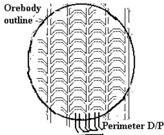
Another area that needs attention is perimeter of a horizontal layout where drawpoints should face outwards so that they draw into caved ground and not that the major apex can be loaded by toe stresses or wedges as shown in the following diagram.
