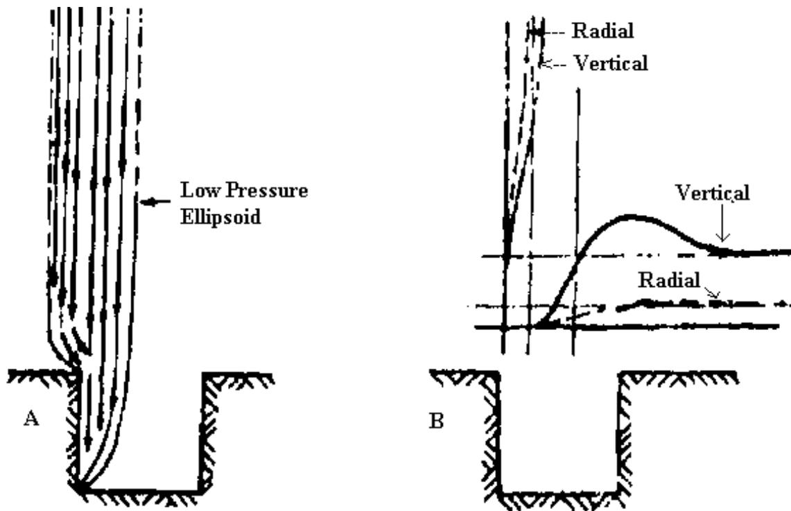
**Flow lines and inferred stress around an isolated working drawpoint**
