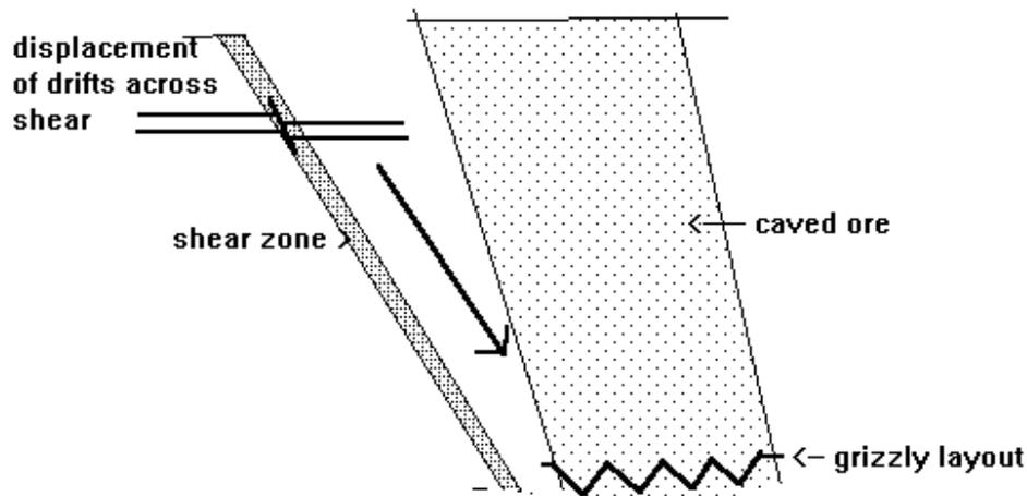
This behaviour can be used to advantage in order to draw ore sitting on a footwall shear:
