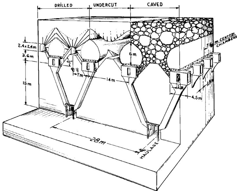
Fig.1 CAVING STEPS AND DESIGN DIMENSIONS OF THE GRIZZLY METHOD
