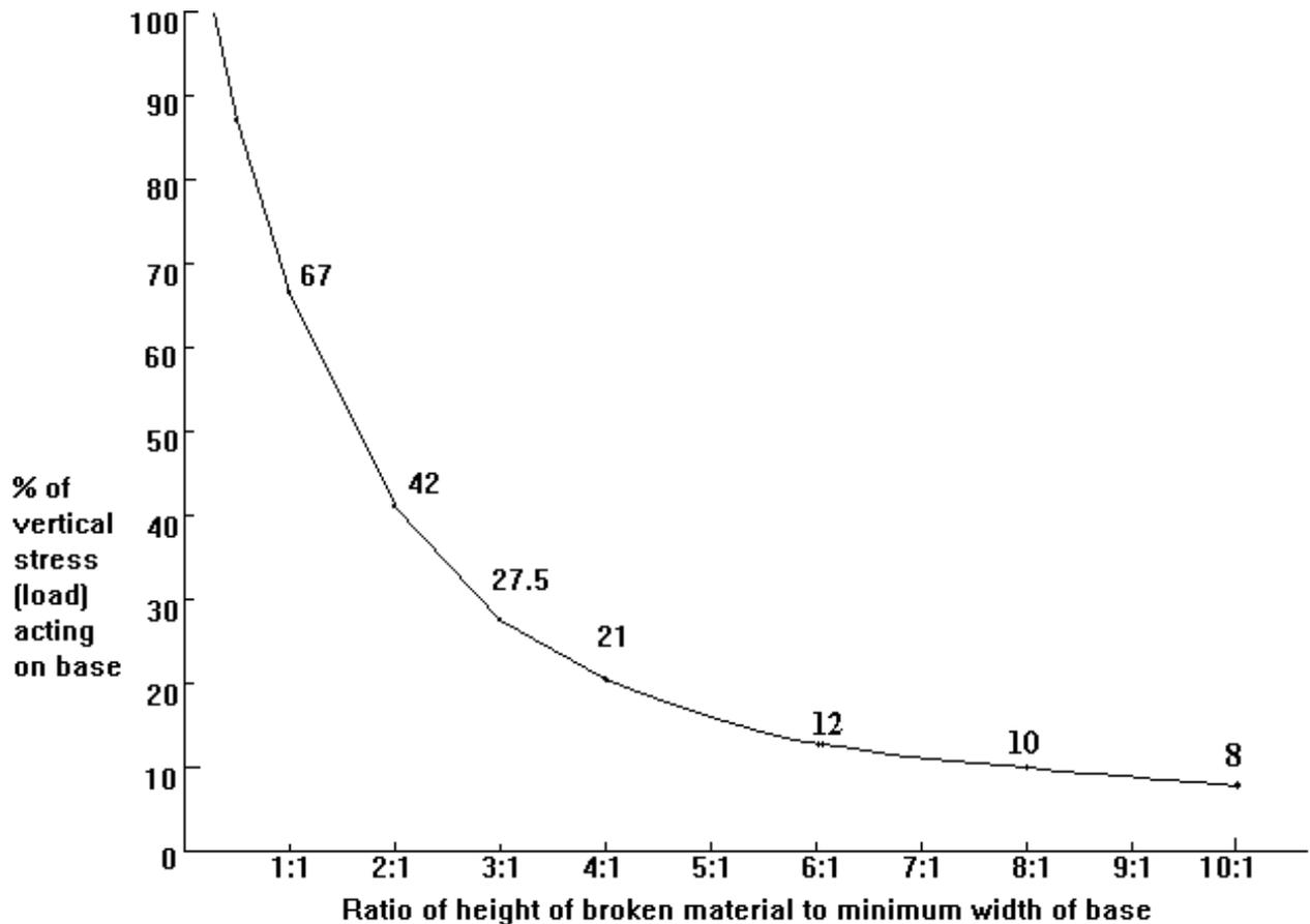
The load on the base should be higher in the centre of the mining area than on the sides.
