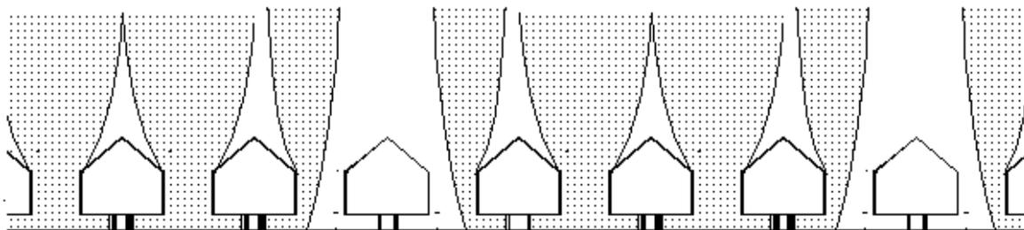
Extraction drifts available for drilling, blasting and repairs on an alternating daily basis
