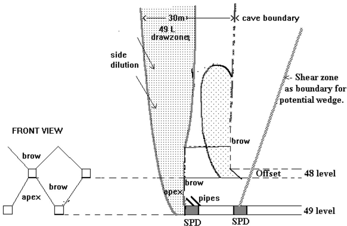
A diagram showing a two level layout with SPDs on 49 level at 15m spacing. 48 level is the undercut level with caving occurring with a 15m face advance. The diagram shows a major shear zone which will form the boundary of a large wedge which would cause extensive damage on 49 level. In this case 48 level would be advanced through the shear zone and the wedge destroyed by undercutting and drawing.
