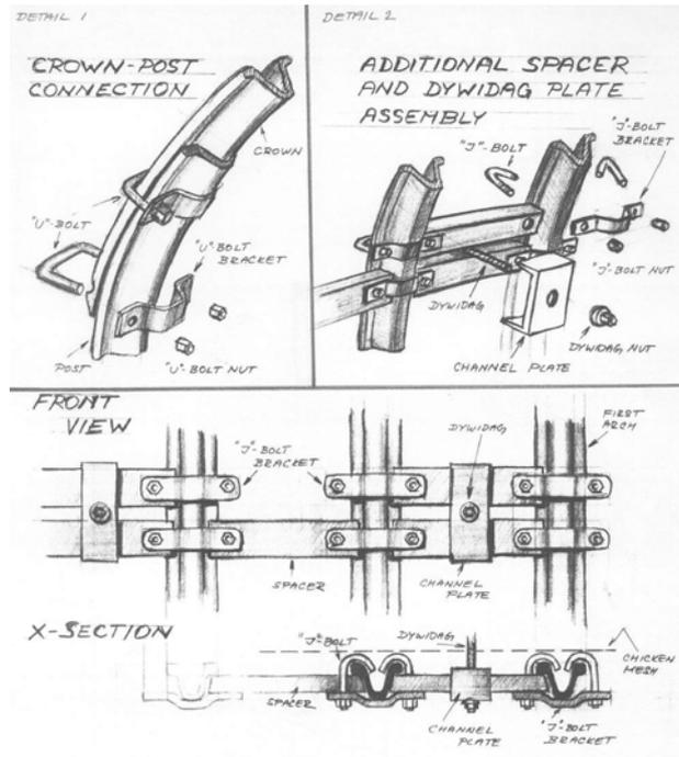
Figure 7a : Connecting channels and 'J' bolts of yielding arch
