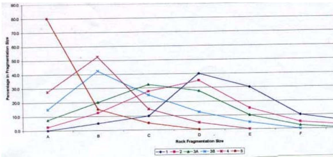
It will be noted that class 3 IRMR has been split into 3A and 3B as they tend to behave differently. 3B ground tends to break and flow and generally behave more like class 4 while 3A ground tends to report as hard pods.
