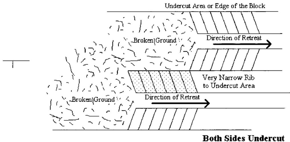
In Shabanie Mine's horizontal undercuts it has been found that single side blasting proved the easiest to manage as the previous development was used and available as an anti-socket drive and to reduce the chances of remnant pillars being formed.
