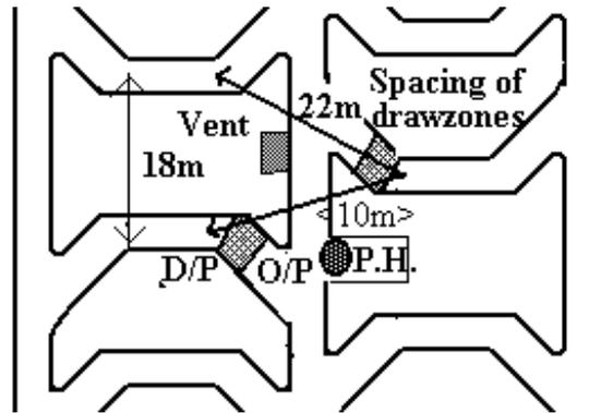
Another factor in favour of the staggered layout is that the drawzone spacing diagonally across the major apex is 22m compared to 27m with the opposite layout.
