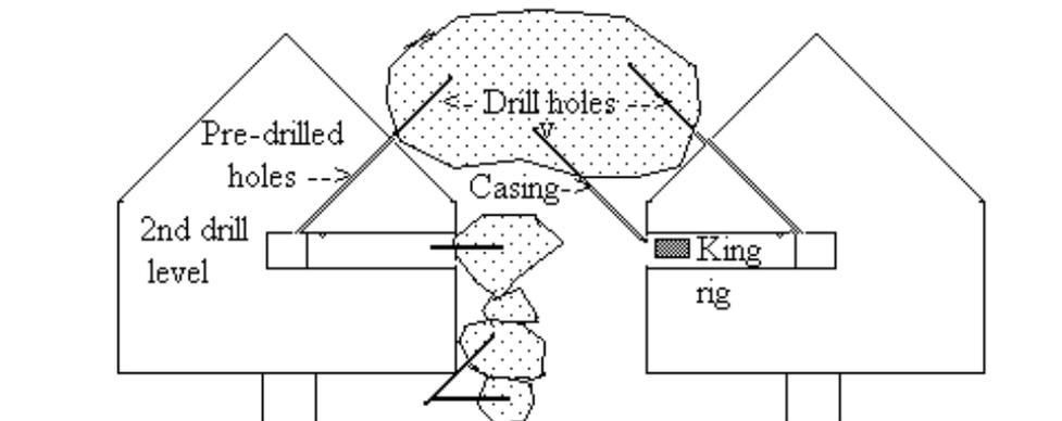
**The secondary drilling level becomes an exhaust airway after the blast, thus clearing the production drift of gasses in a very short time.**
