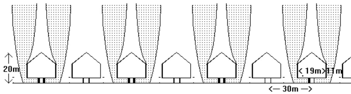
Figure 2 A - draw pattern of drawpoints either side of major apex i.e. from extraction drift
