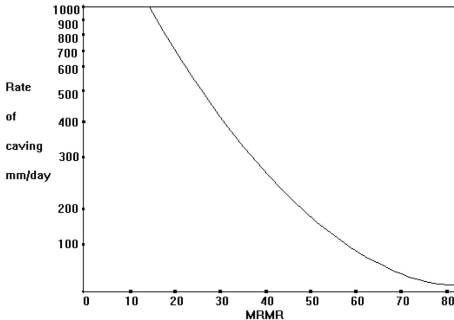
**DRAW RATE LESS THAN RATE OF CAVING TO ENSURE THERE IS NO SEISMIC ACTIVITY IN THE CAVE BACK**
