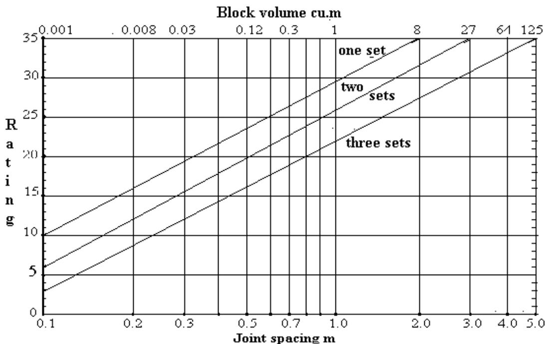
Figure 6. Joint spacing ratings
