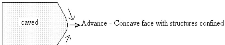
A convex face is less stable both in the cave back and on the undercut and production levels.
