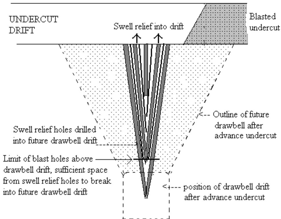
A possible problem is that owing to the V shape the broken rock will arch and not flow into the drawbell drift when it intersects the base of the winze. There could be sufficient relief for the adjacent ring holes to be blasted. However, if this is a permanent problem then a vertical winze might be required. Also the blasting could be done from the drawbell drift when it is developed. In weak rock or high stress areas it would be best to blast as a blind winze.
