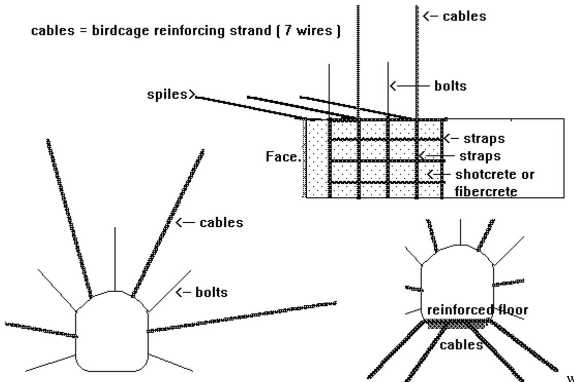
Polystyrene / Styrofoam models should be used to display the bolt patterns to determine if the coverage is sufficient. The drifts are modelled as the solid and the bolts cut to the right length from coloured blasting wire and inserted into the model. The end result appears as loaves of bread resembling a porcupine.
