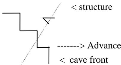
The cave front must be at a fairly large angle to the access drift as it moves across it to minimise abutment stress effects:
