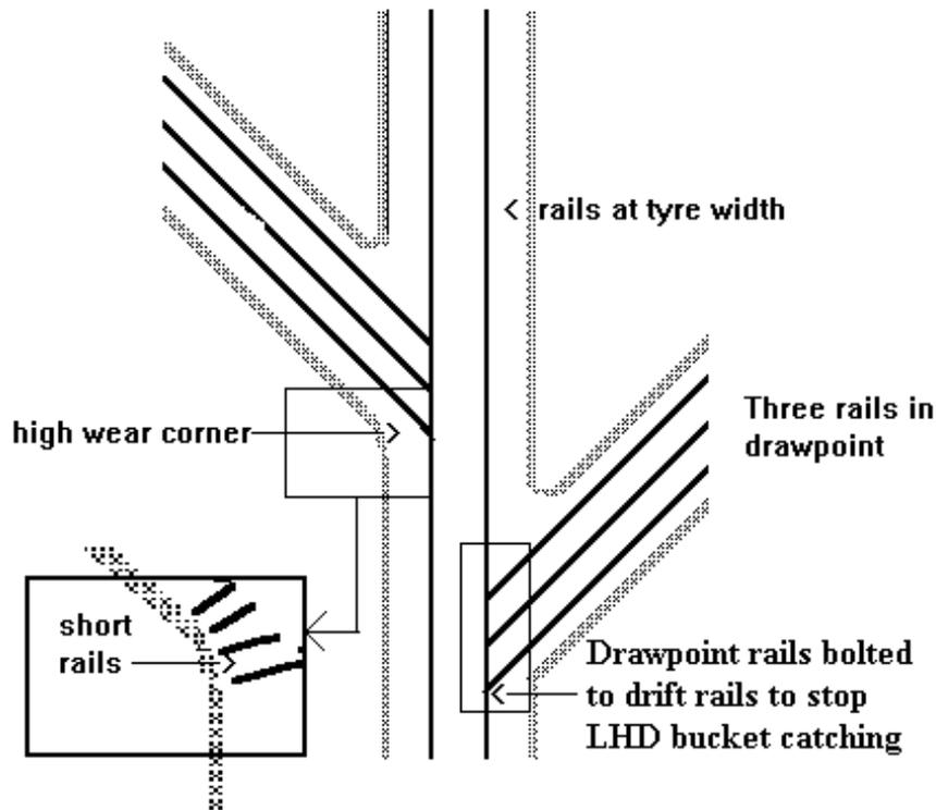
**Rails embedded in concrete to stop wear and to assist the cleaning of the drift.**
