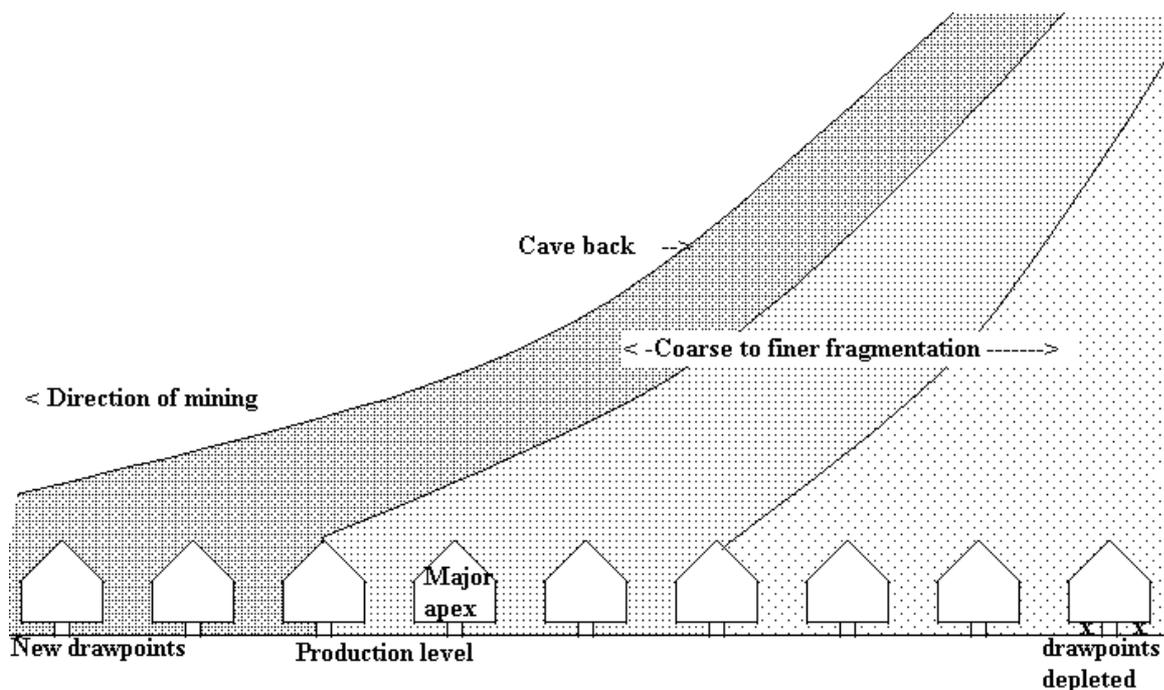
This is a continuous operation which makes production scheduling simpler. It is essential that an air gap is not allowed to develop otherwise there can be migration of material down the cave back, as this could lead to the early introduction of dilution.
