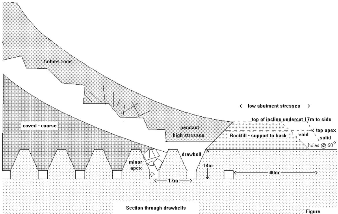
**Undercut drifts** -The following diagram shows two layouts one with the undercut drifts developed on two levels and the other on the same level. A drift is developed over the top of the major apex to provide a check on the accuracy of the drilling and also as an anti - socket drift. The long hole drilling is done from the drift over the drawbells and in the diagram 20m holes are envisaged, with modern drilling equipment this is no problem.
