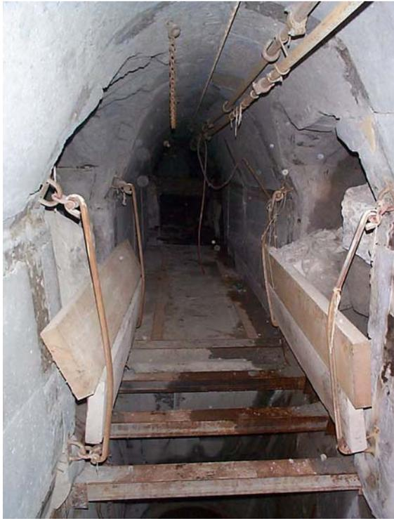
**View down a grizzly drift in early stages of draw. The opposite drawpoints with boards in place to control the gravity flow into the central orepass**
