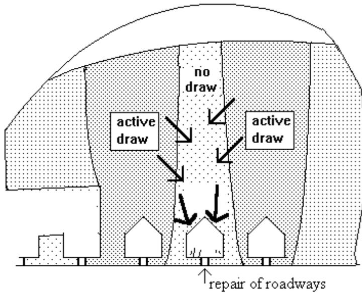
Weight of broken ground plus the arching stresses of the adjacent drawzones imposes a significant load on the major apex and thus on the pillars of the extraction horizon.
