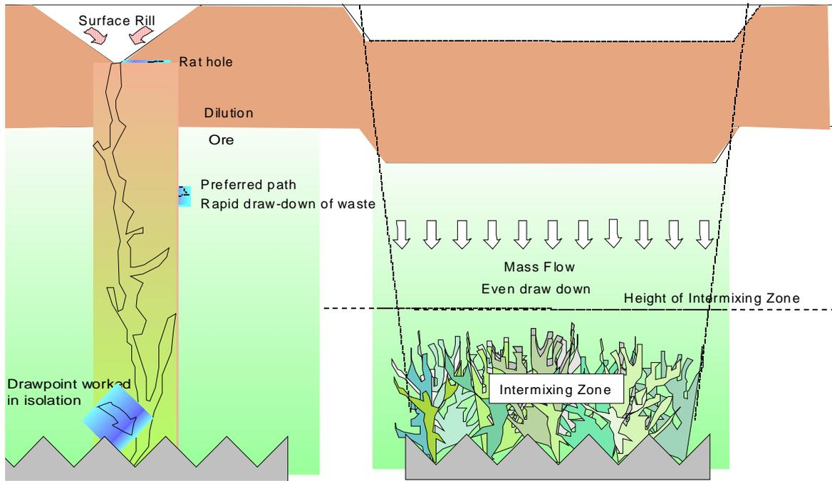
**Figure 6** Void Diffusion (VD) mechanisms – The formation of preferred channel leading to rat-holing for a drawpoint worked in isolation (left) and overlapping of multiple “palm and finger” drawbodies when drawpoints worked concurrently (right).
