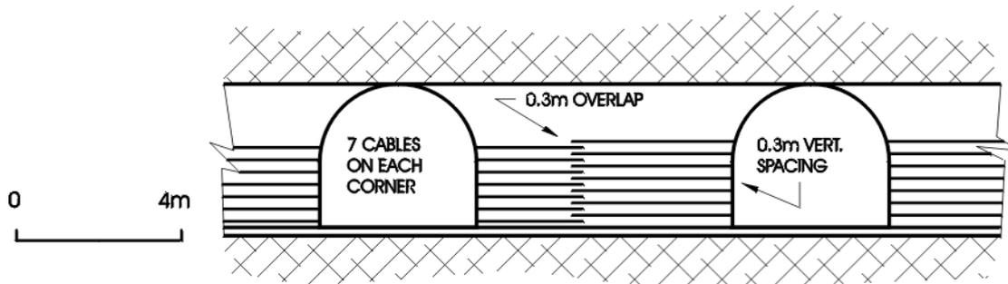
Bullnose and camelback support in potential squeezing ground
