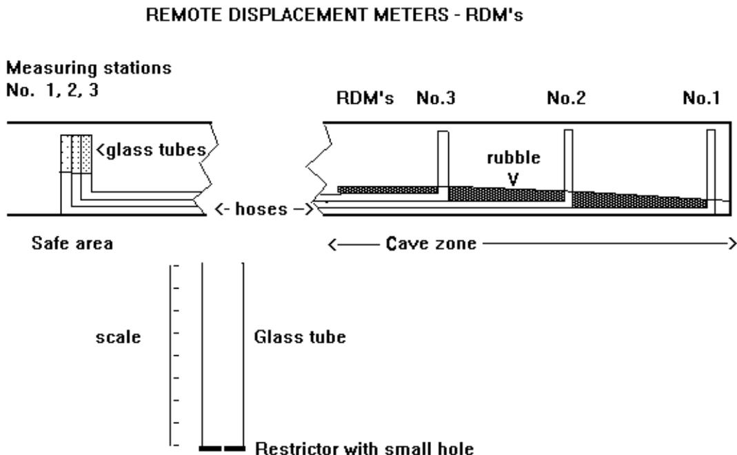
These devices can also be placed in shallow upholes, the inclination of the holes will depend on the elevation of the measuring site. If a drill hole raise is available then the hole can be steeper or longer.
