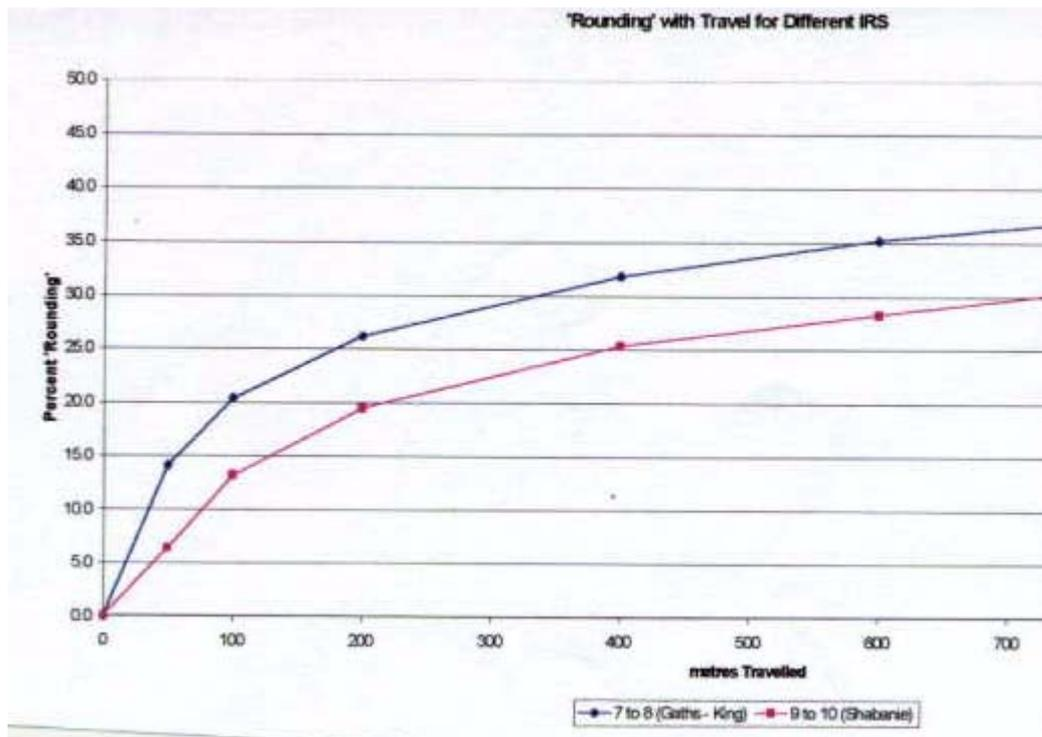
The rounding will produce fragments that are two and three rock sizes below the block from which they came see tabulation below. The ratio of smaller fragments will be approximately half each.
