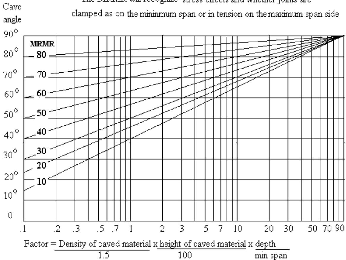
The above diagram is a conservative approach and should be used for siting important infrastructure such as shafts or plant.
