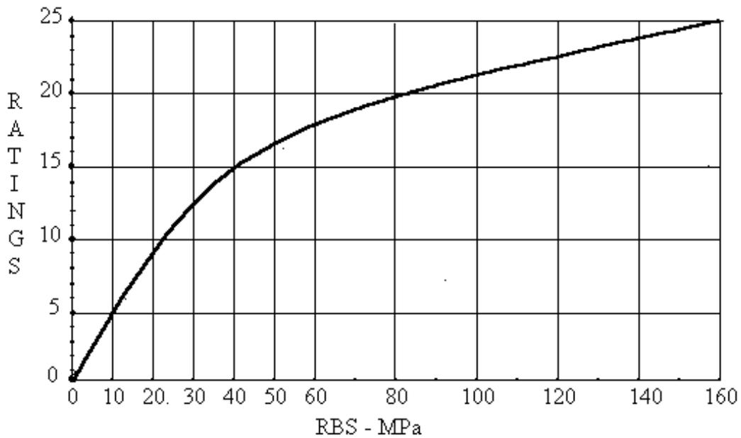
Figure 5. Rock block strength rating as a function of rock block strength.
