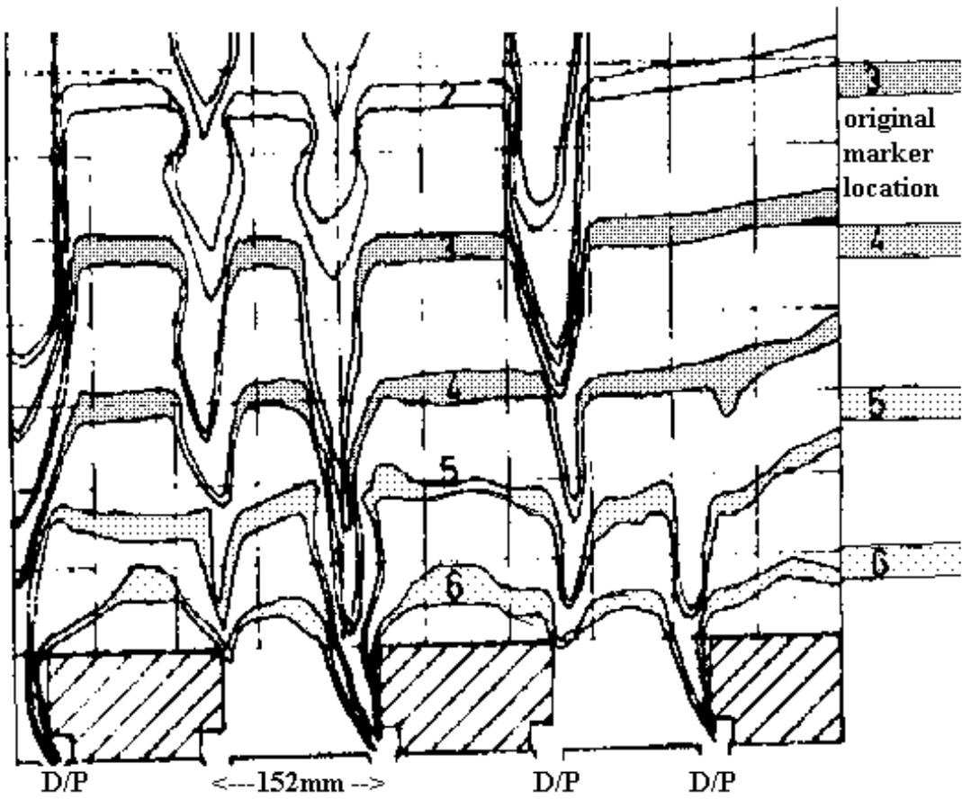
Lateral stresses in the induced stress zone surrounding a draw column is possible if the vertical pressure is further increased by working adjacent drawpoints.
