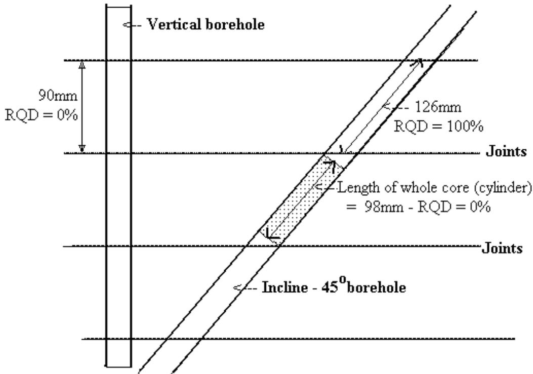
**Difference in RQD for an angled versus a vertical borehole**
