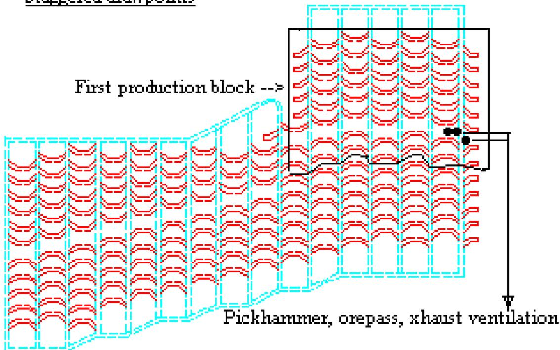
The details of the staggered mirror image herringbone layout are shown in the following drawing:
