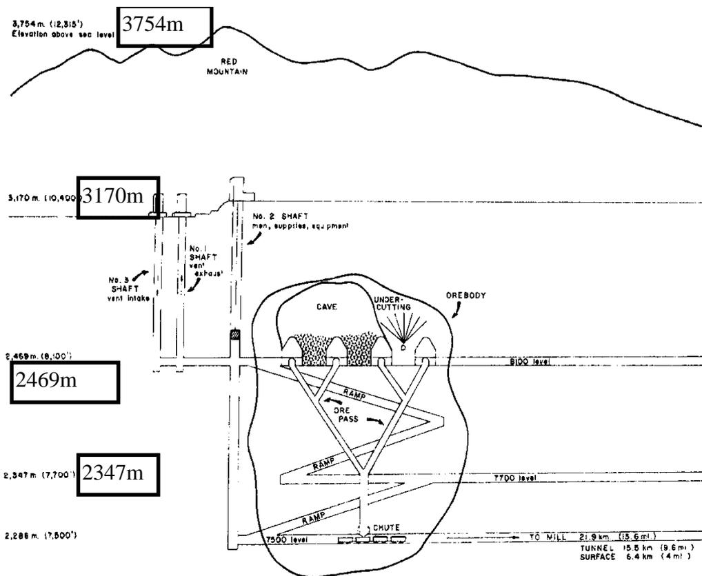
Figure 2. Generalized section, Henderson Mine.
