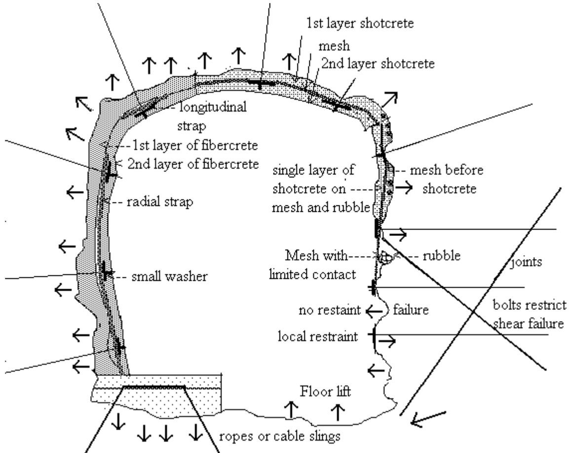
**Early installation of full rock reinforcement will result in a sound support system**
