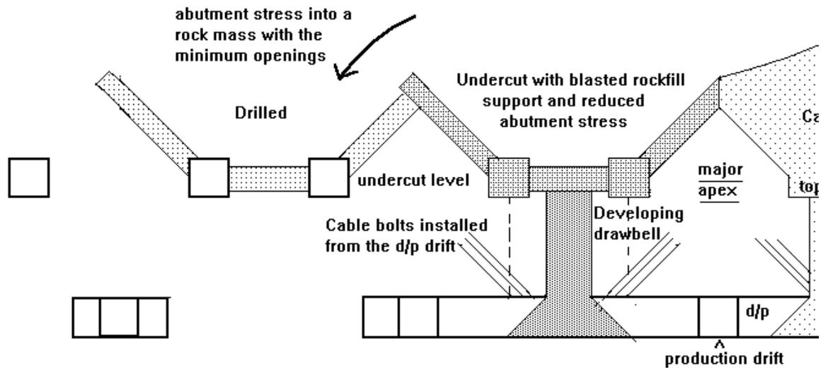
**INCLINE NARROW ADVANCE UNDERCUT SEQUENCE WITH CABLES INSTALLED FROM DRAWBEL**
