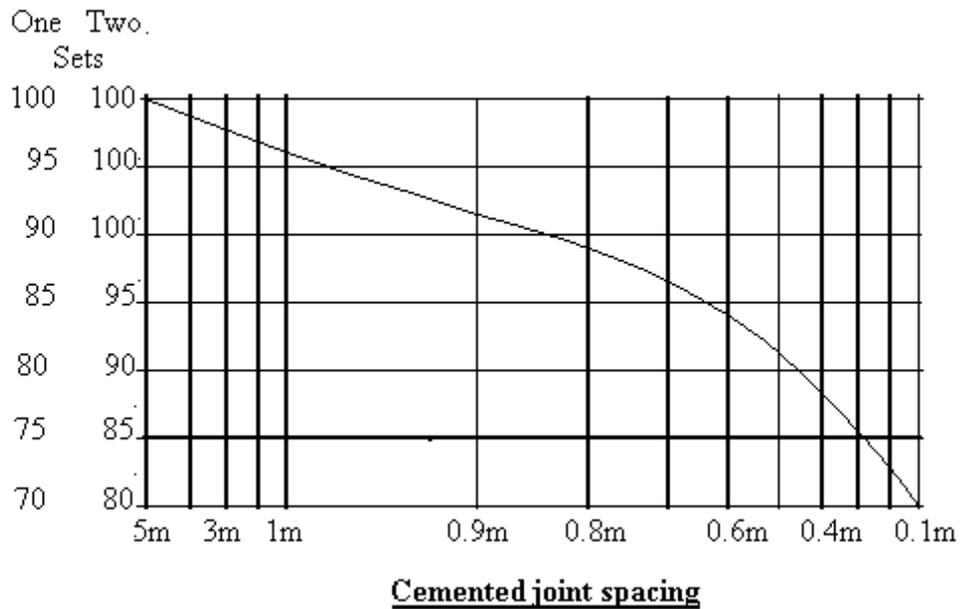
Figure 7. Adjustment factor for cemented joints
