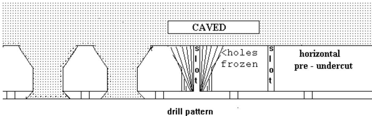
The shape of the major apex could be checked by drilling from the production drift through the major apex.
