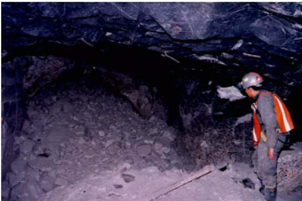
In the conventional layout it is common for the pillars to show a high degree of fracturing after the undercut has passed, these 'pillars' only represent 50% of the solid rock on a production level, the fracturing most likely means that the solid core of the pillar is about 20% of the area and hardly sufficient to withstand any traumatic event. A combination of poor draw or a seismic event could set up a domino effect.
