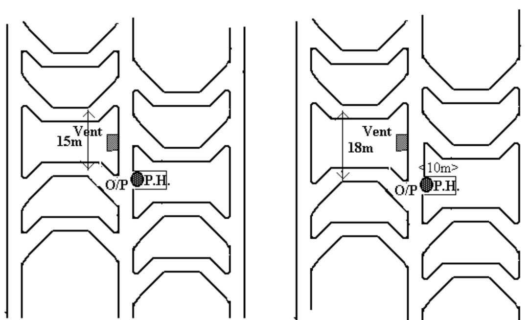
The staggered layout is better in terms of pillar location with respect to the shape of the orebody and the offset of the pickhammer and the ventilation raise results in a stronger layout.
