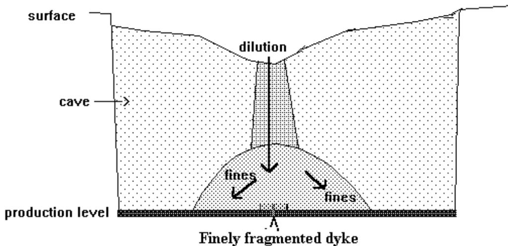
**Preferential draw of fines into central drawpoints with more rapid lowering of the surface in the centre and rapid infiltration of the dilution**
