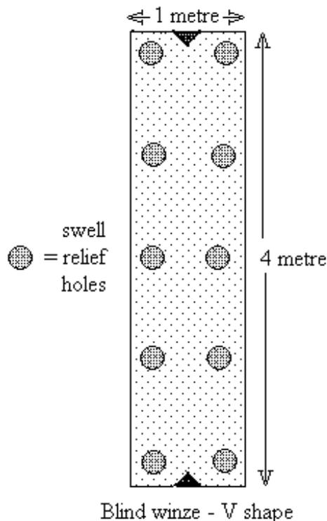
Plan above and section below of a V shaped blind raise drilled and blasted from the undercut drift in close proximity to the undercut blasting. The actual timing has to be sorted out, but it could be concurrent with the adjacent undercut blast, if some blasted rock has been loaded.
