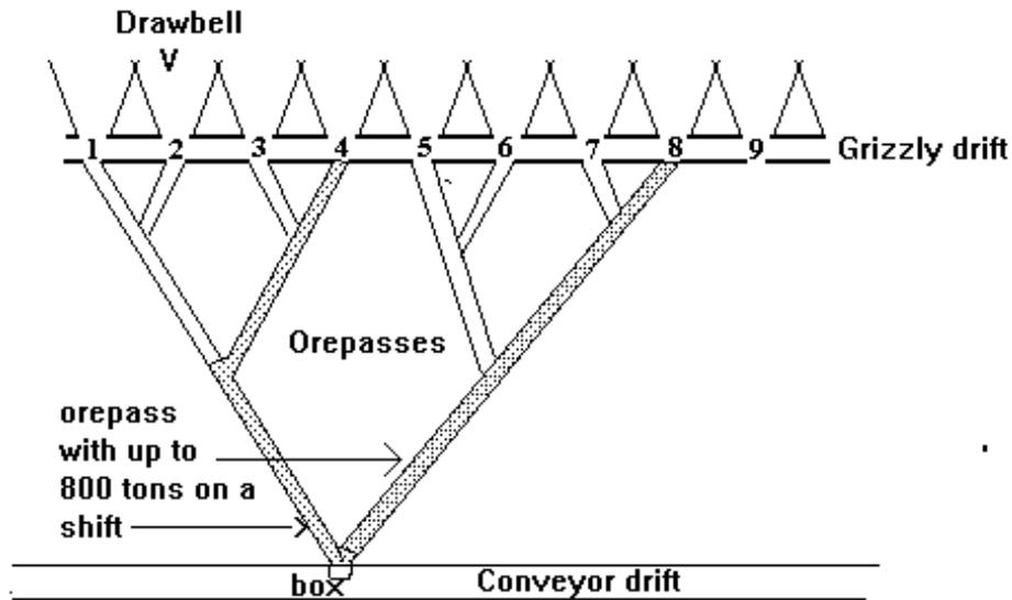
The solution to the problem is to have short orepasses, a flow control at the drawpoint and a fairly uniform draw. Where this is the case, because of the close spacing of the drawpoints, the ore recovery is good and dilution is low.
