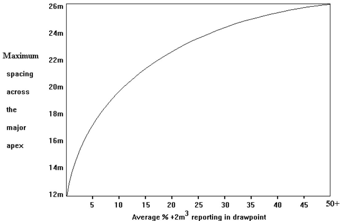
Examples of maximum spacing relative to the +2m<sup>3</sup> content for different mines is shown graphically overleaf. Extra curves have been put onto this graph to indicate other factors which will influence the flow of caved material:
