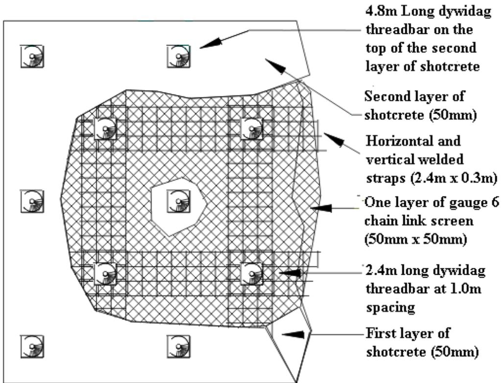
**Installation sequence to obtain a sound rock reinforcement system**
