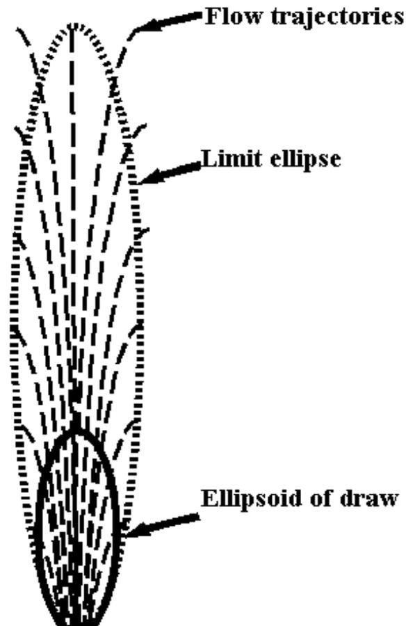
**Figure 1** Kvapil's "Gravity Flow" ellipsoid of draw (the amount of material drawn out), the limit ellipse, i.e. the limit of disturbance when the ellipsoid of draw is withdrawn, and the particle flow trajectories.
