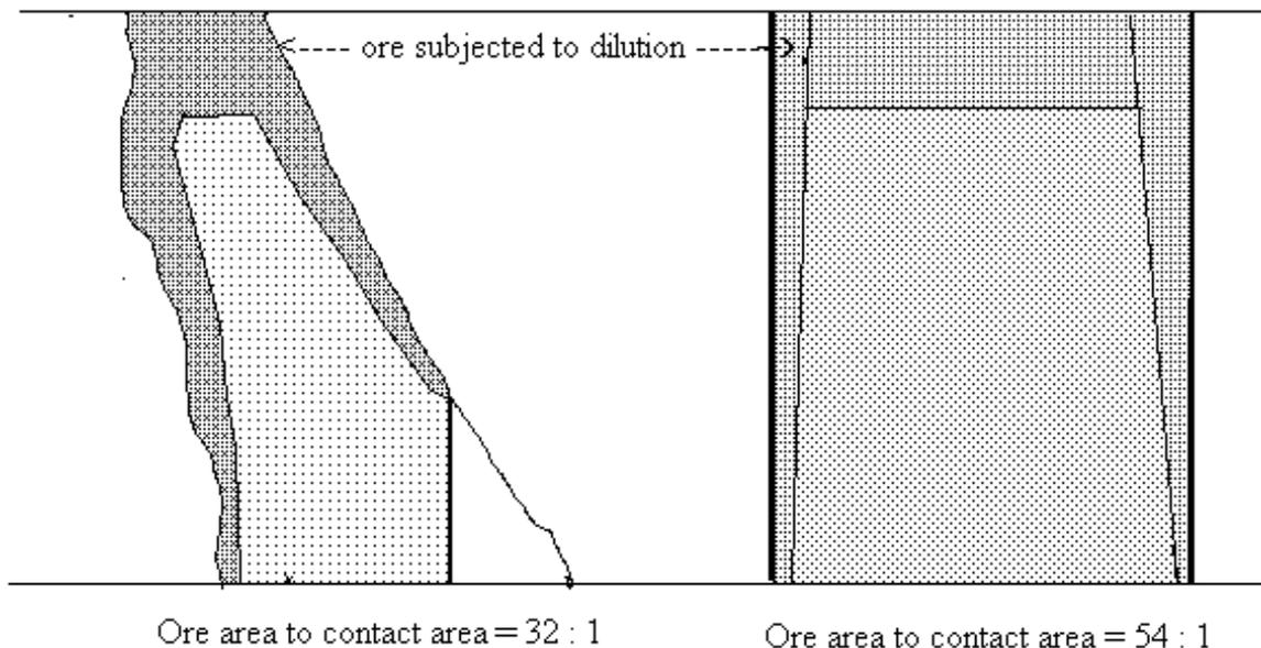
In the above example, the diagram on the left shows a large percentage of the ore is liable to dilution while there is a significant difference between the ratios of the two diagrams. As the orebody become wider the side dilution becomes insignificant.
