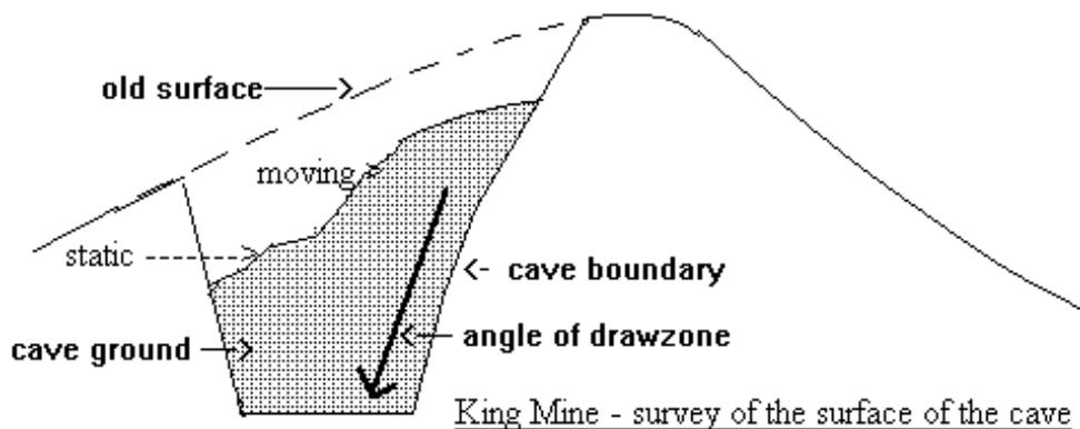
It was noted during the course of surveying the cave surface that the area vertically above the bulk of the drawpoints was static, whilst the slope against the hill was moving down. This implied that drawpoints need only cover half the orebody to recover the ore on the hangingwall side of the orebody.
