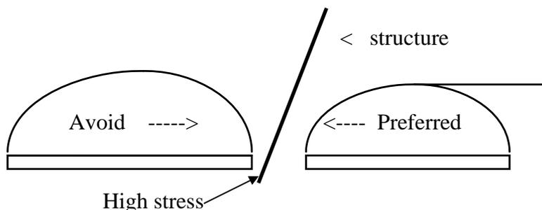
If possible, the cave front should not be advanced towards structures that could initiate massive wedge failures. However, if the cave front has to advance towards major structures these should be crossed at as large an angle as possible:
