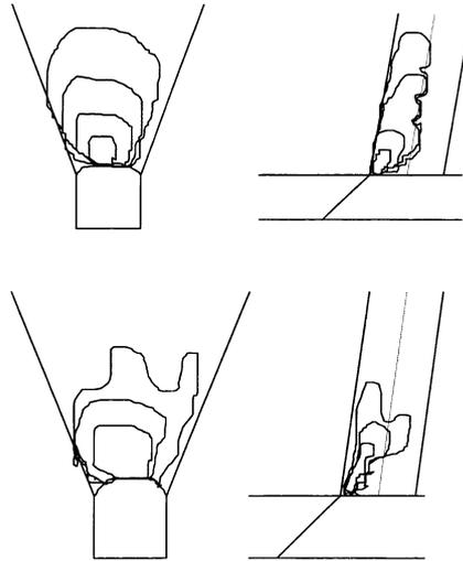
**Figure 3** Gustafsson's "palm and finger" drawbody shapes from full scale marker experiments at Kiruna Mine
