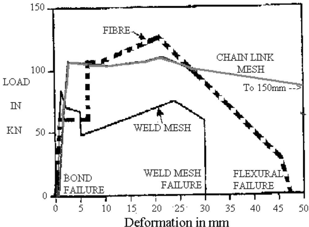
A factor which is ignored in these tests or possibly not emphasised is the proportion of steel in the reinforcing. There are published results comparing a 4% fibre content with shotcrete with 1.4% mesh.
