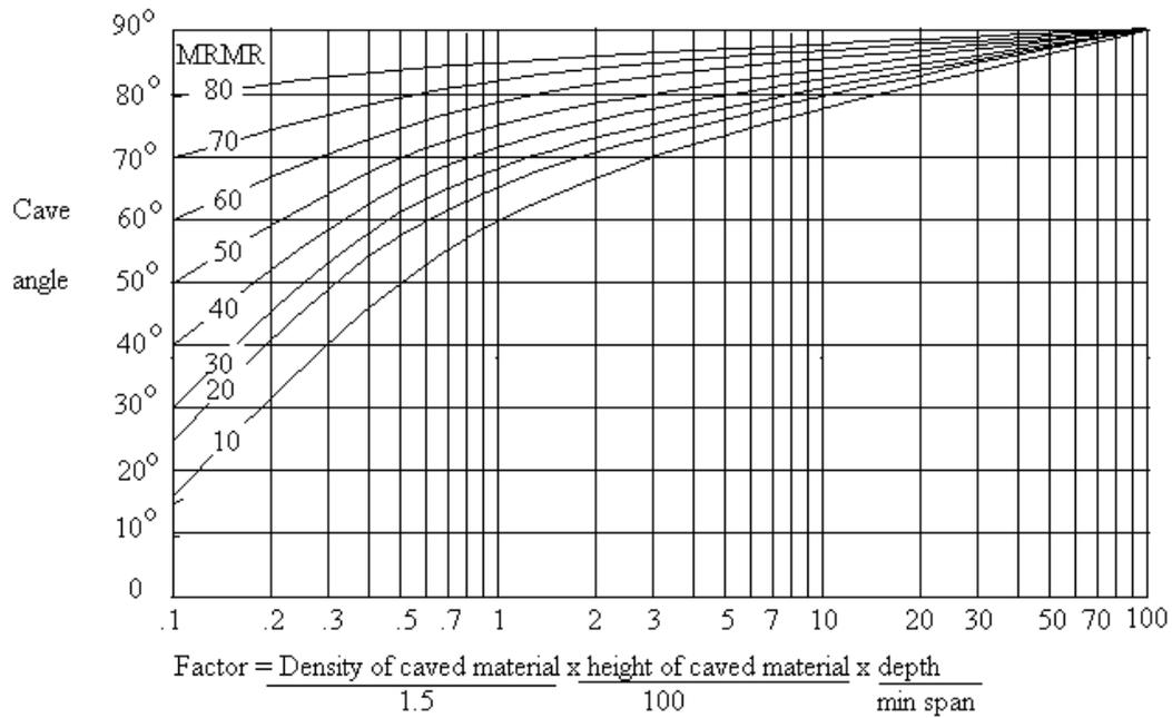
The above diagram is less conservative and would be used for draw control and water inflow calculations.
