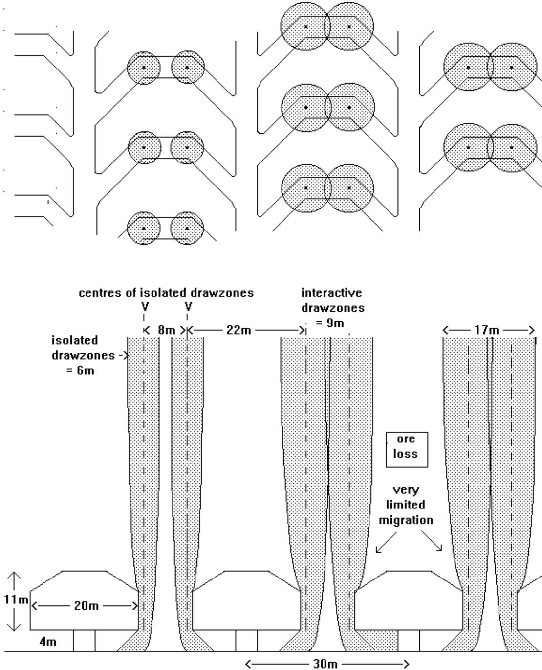
Fine - medium fragmentation +2m<sup>3</sup> = 2% to 9% - interaction poor
