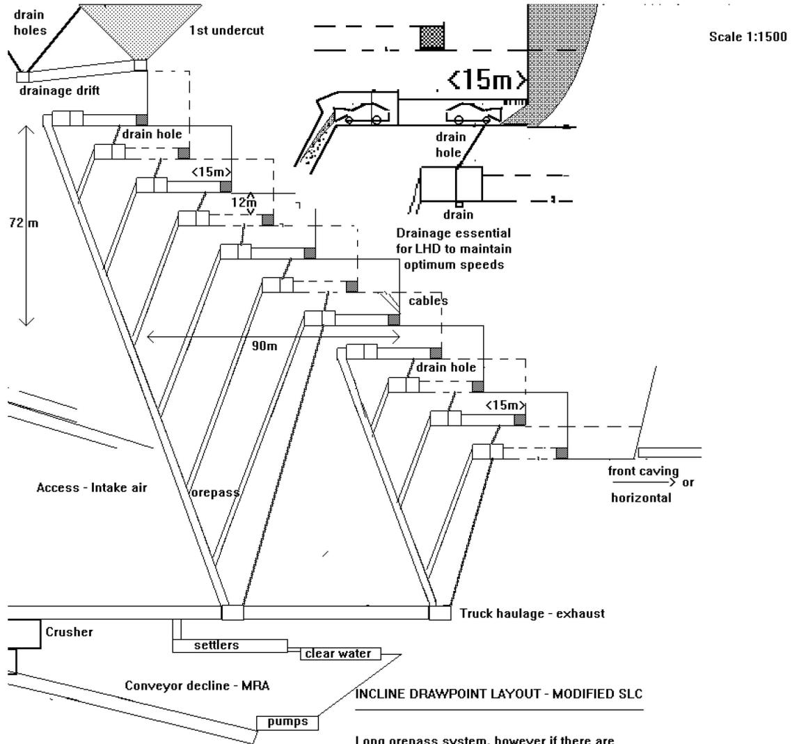
Long orepass system, however if there are likely to be hangup problems due to mud or packing then orepasses will be shorter and collecting levels are required - see Batu 1.
