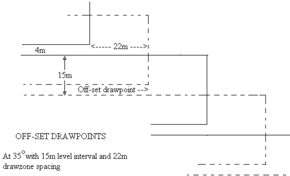
Thus the spacing from level to level can be 15m, from drawpoint to drawpoint on the level from 12m to 15m depending on pillar strength and from level to level it would be 22m which would relate the 22m across the major apex in some horizontal LHD layouts.
