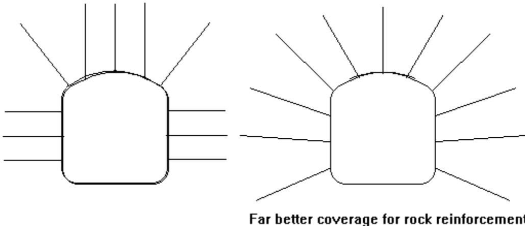
The practice of increasing the bolt spacing in more competent the ground is common. As the object of the exercise is to ensure that blocks do not fall from the back then this approach is not correct as widely spaced bolts will not cross widely spaced joints and will be contained within the large rock block. Also bolts at 1m cover 1m<sup>2</sup> whereas a bolt at 1.5m spacing covers 2.25m<sup>2</sup>.
