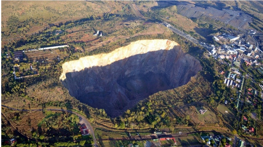
Figure 12. The pit at the Premier Mine, Cullinan, Gauteng, South Africa. The cross-sectional area of the 190 meter deep pit at its surface is about 32 hectares. The mine was the source of the 3106 carat Cullinan Diamond, the largest diamond ever found.
