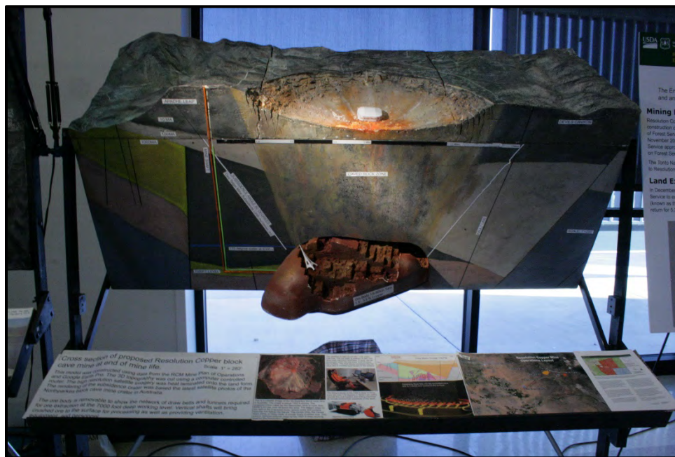
Figure 2.3.4.7-2. Photo of model section 2; cut-out view of subsidence crater and ore body.
