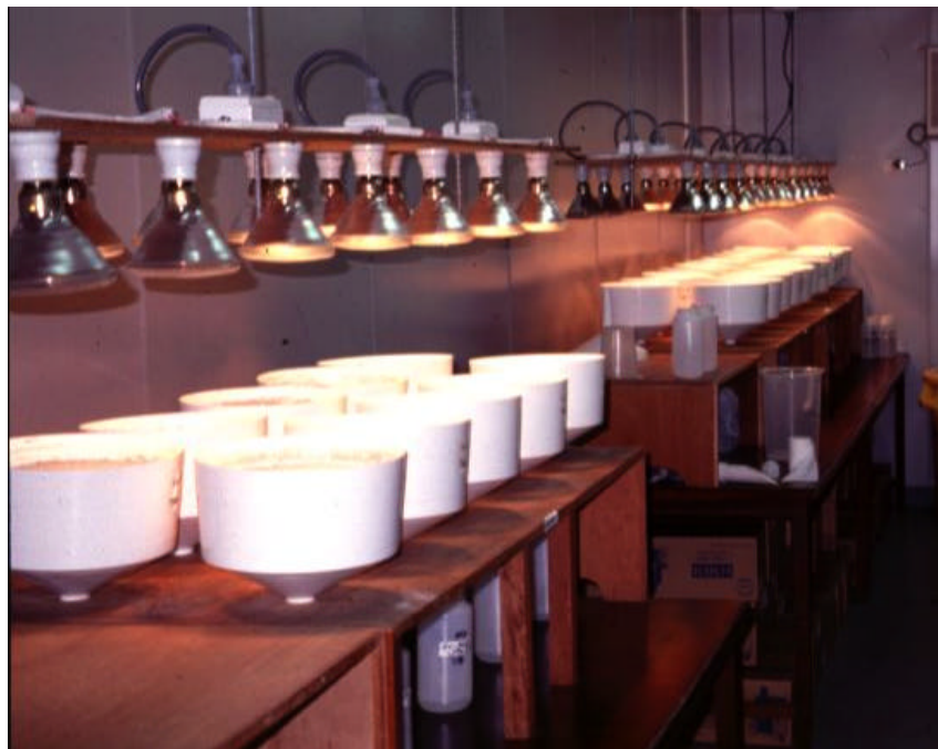
Plate F1: Free draining leach column test set-up using Buchner Funnels.
