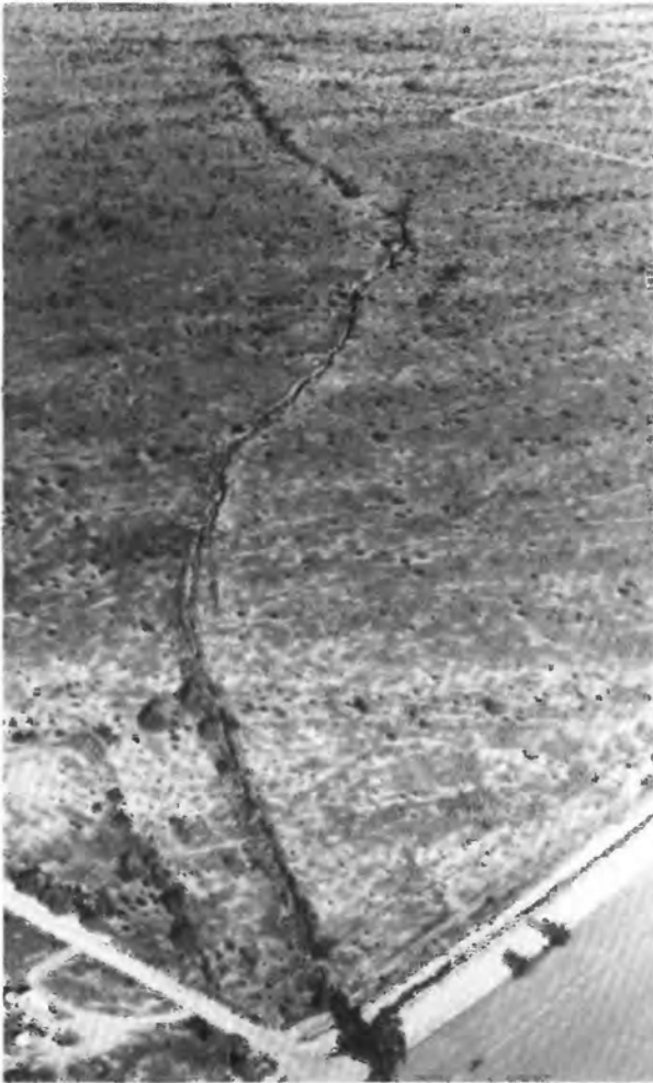
FIGURE 27.—Earth fissures and effects of land subsidence in alluvial basins near Eloy and Phoenix, Arizona.
