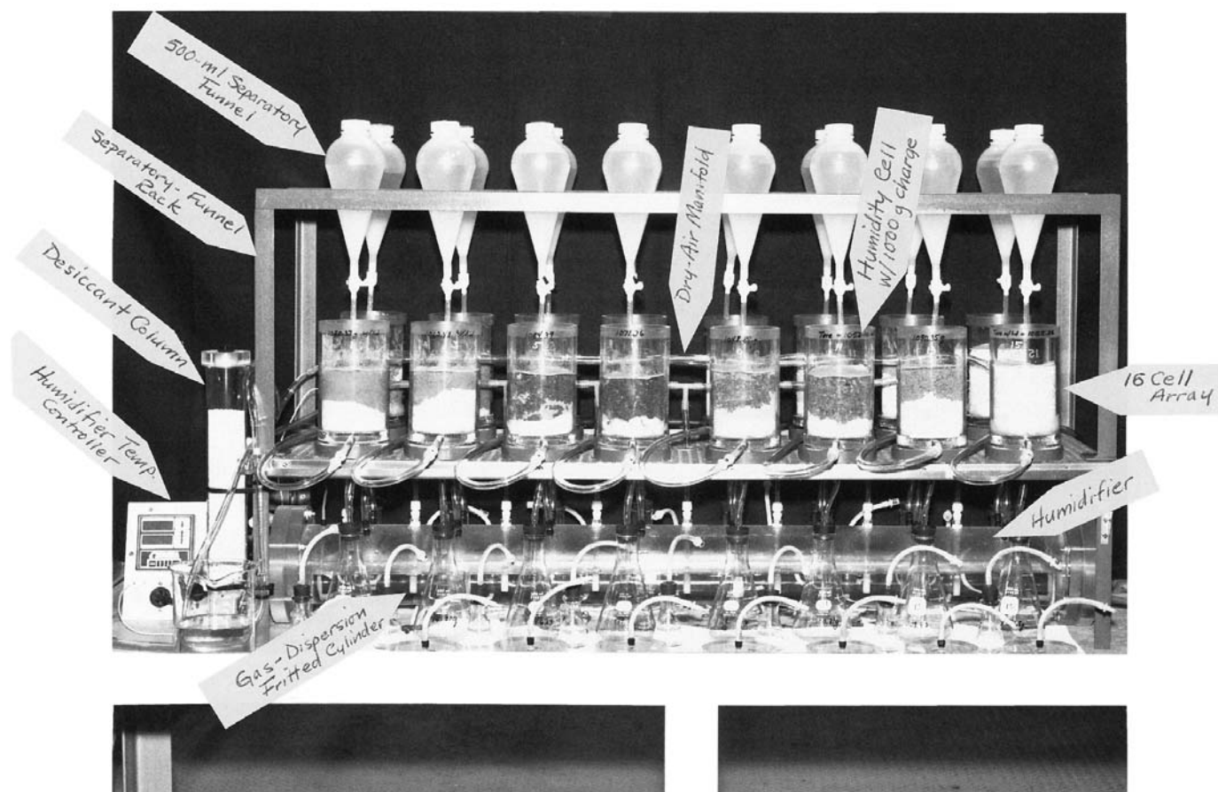
FIG. 2 Front View of 16-Cell Array with Separatory Funnel Rack
