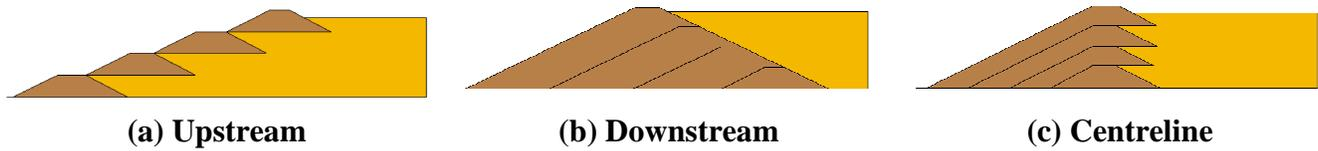
**Figure 3: Broad types of methods for raising tailings dams**
