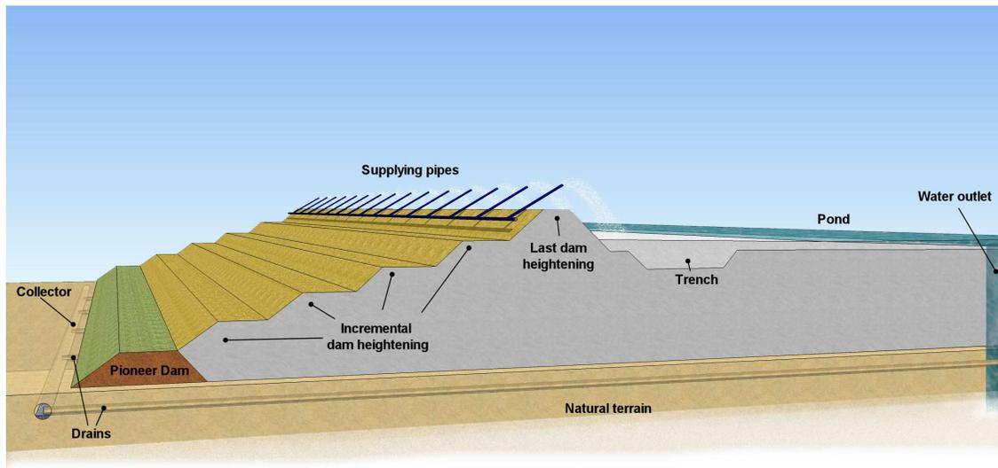
**Figure 2: Example of tailings dam profile**
