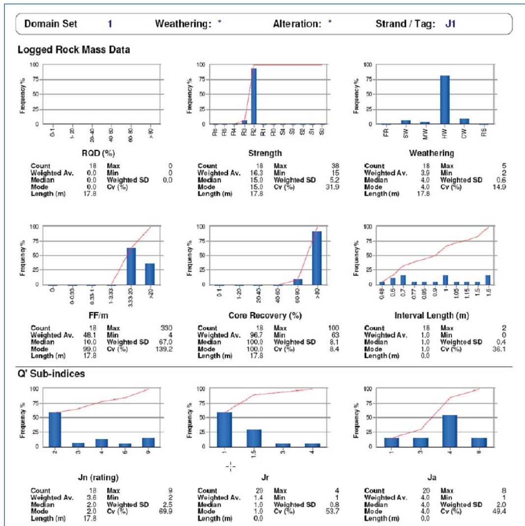
Figure C1. Example output from acQuire. Data entry panels (top graphic), simultaneous down-hole charts (center graphic) and statistical analysis graphs (bottom graphic) are designed to help maintain quality of a drill hole database (Pere et al., 2011).
