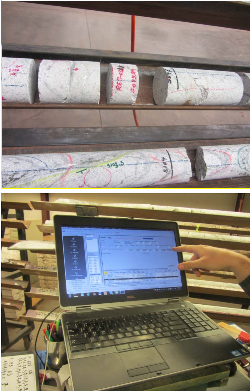
Figure C3. Core being logged (upper photo) and real-time data entry into acQuire software on a laptop at a geologist's core logging station (lower photo). [Brandt et al., 2017; Pere et al., 2011]
