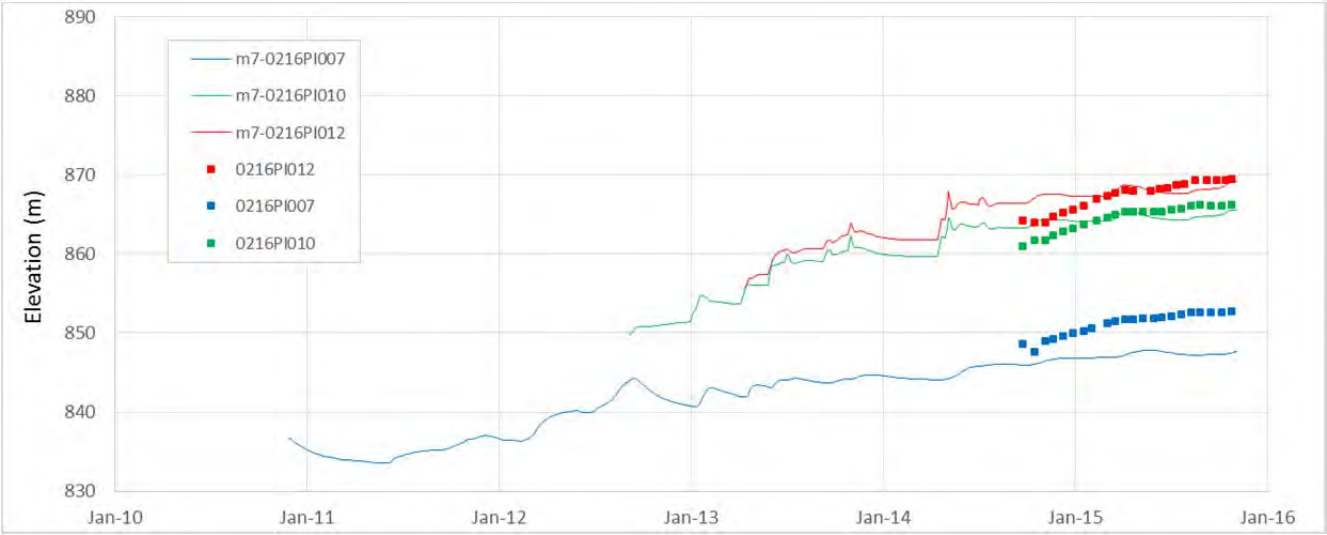
Figure G3-15 Calibrated transient model hydrographs, measured versus modeled, line 02
