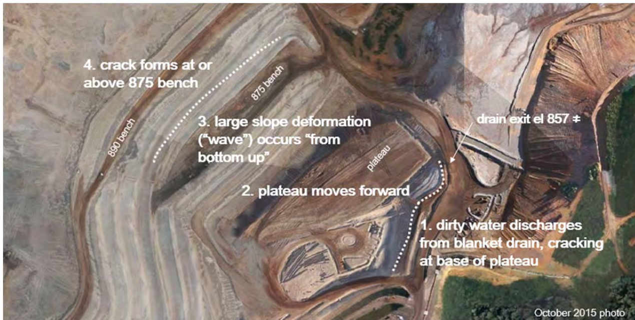
Figure 2-18 Failure initiation sequence
