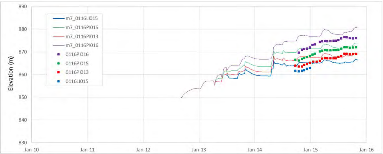
Figure G3-14 Calibrated transient model hydrographs, measured versus modeled, line 01
