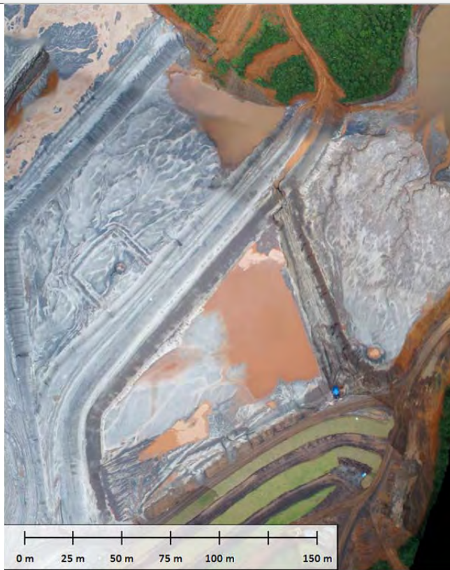
March 2, 2013 Samarco aerial image showing the Secondary Gallery sinkhole to the left and a region of saturation and ponding to the right at the dam's contact with the left abutment.
