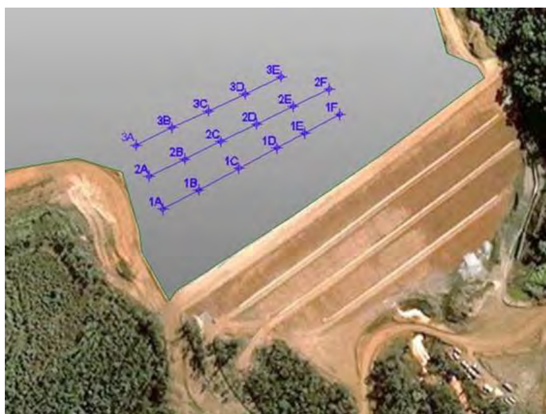
Figure D2-1 Approximate location of sample collections for Campaign 1 at Dike 1 (Figure 3.3, page 41 of thesis)
