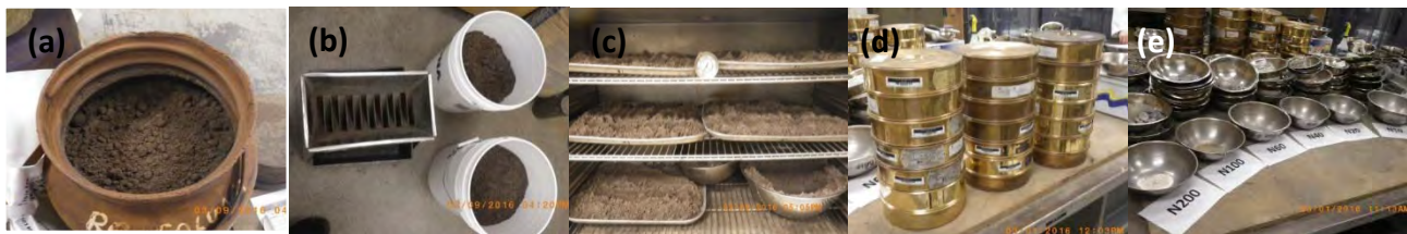
(a) Field sample, (b) Sample mixing, (c) Sample air drying, (d) Sample sieving, (e) Split sample
