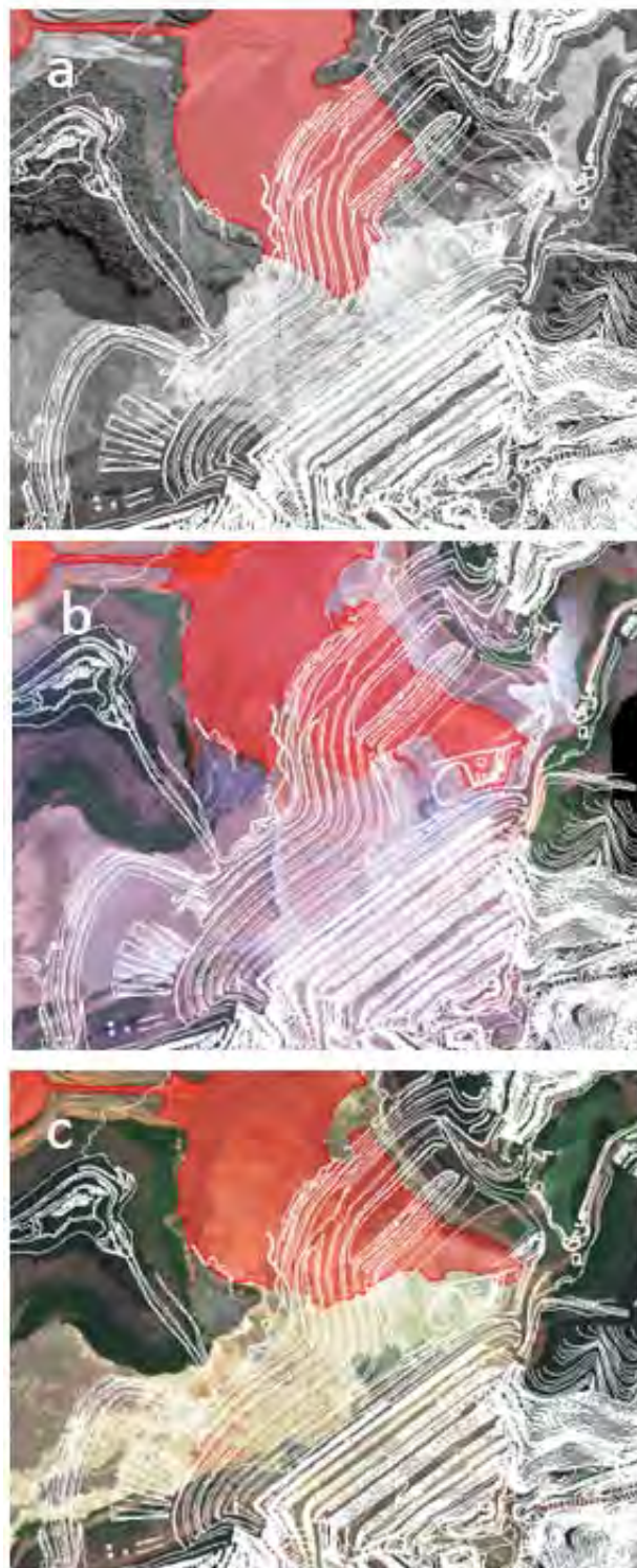
Figure 5-11 Slimes beneath final embankment: (a) September 20, 2011; (b) January 21, 2012; (c) March 3, 2012. Slimes highlighted in red; final embankment contours in white
