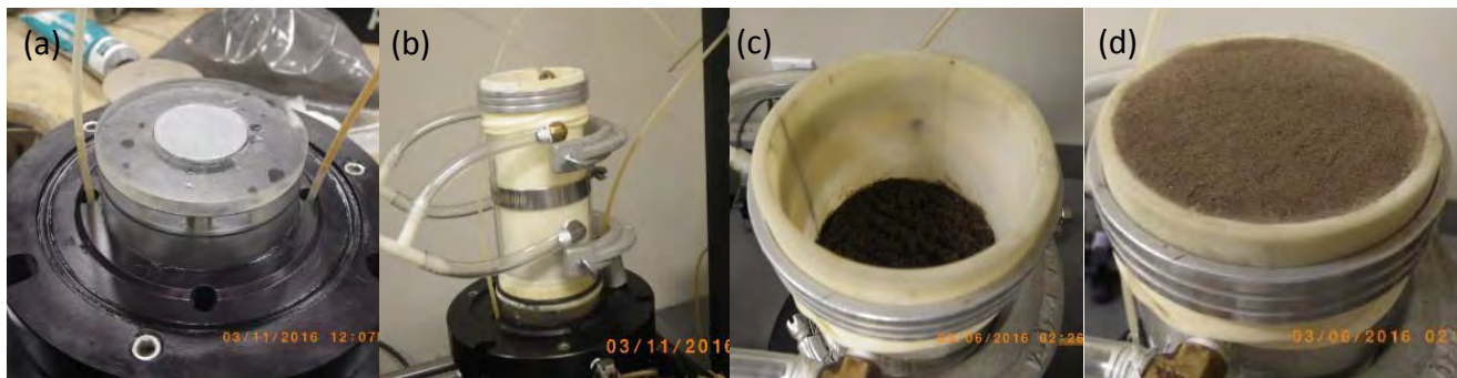
(a) Modified porous stone, (b) Specimen setup, (c) Specimen placement by moist tamping, (d) Final specimen
