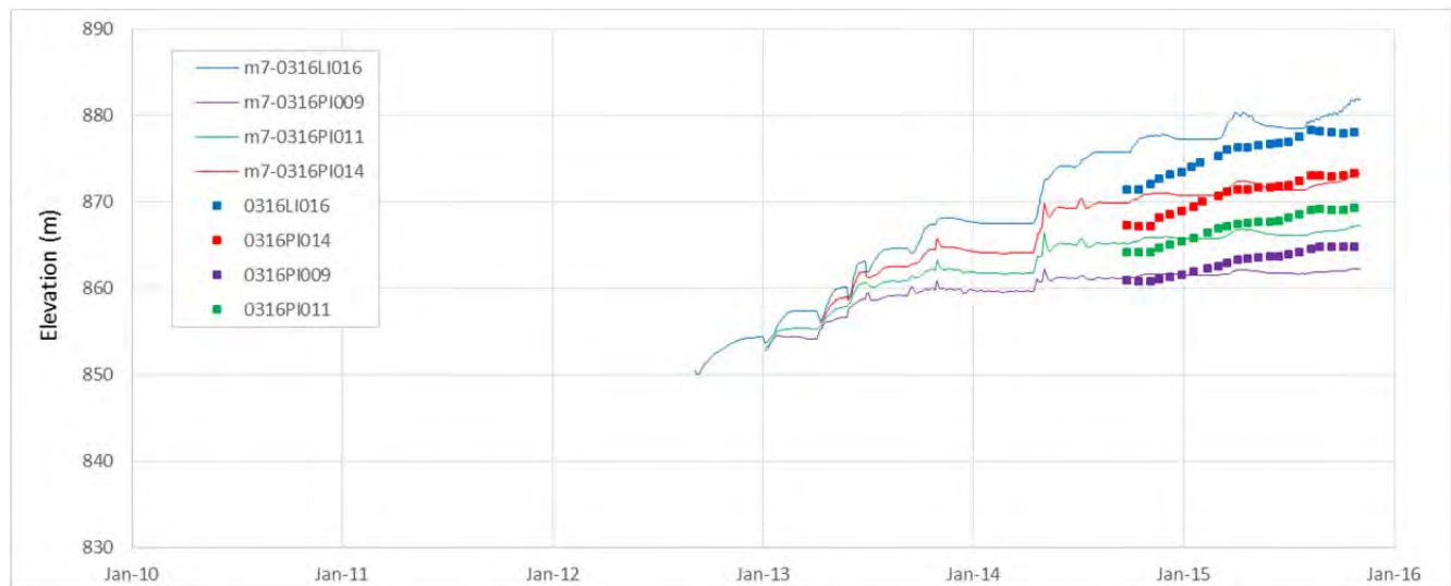
Figure G3-16 Calibrated transient model hydrographs, measured versus modeled, line 03
