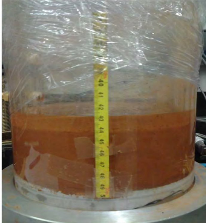
Figure 4. Settlement test conducted in a consolidation cell at the end of the test.
