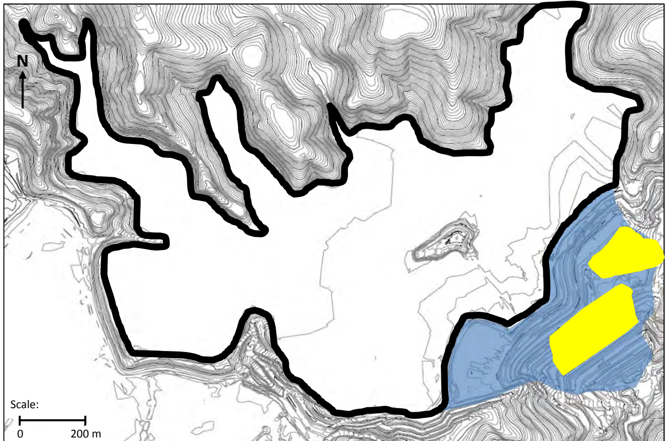
Figure 4-11 November, 2015 configuration showing El. 826 m and El. 860 m blanket drains, raised dam, and impoundment outline
