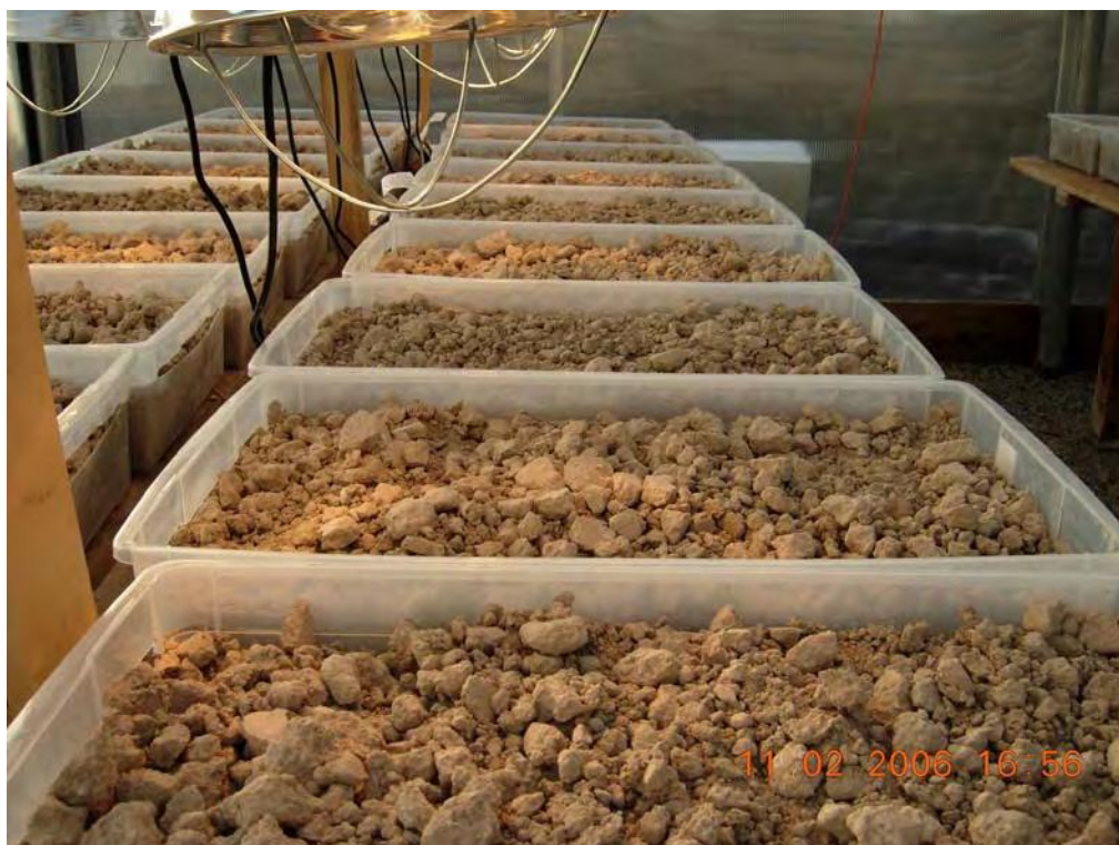
Figure 2-10. Treated Nevada Soil Trays Under the Heat Lamps
