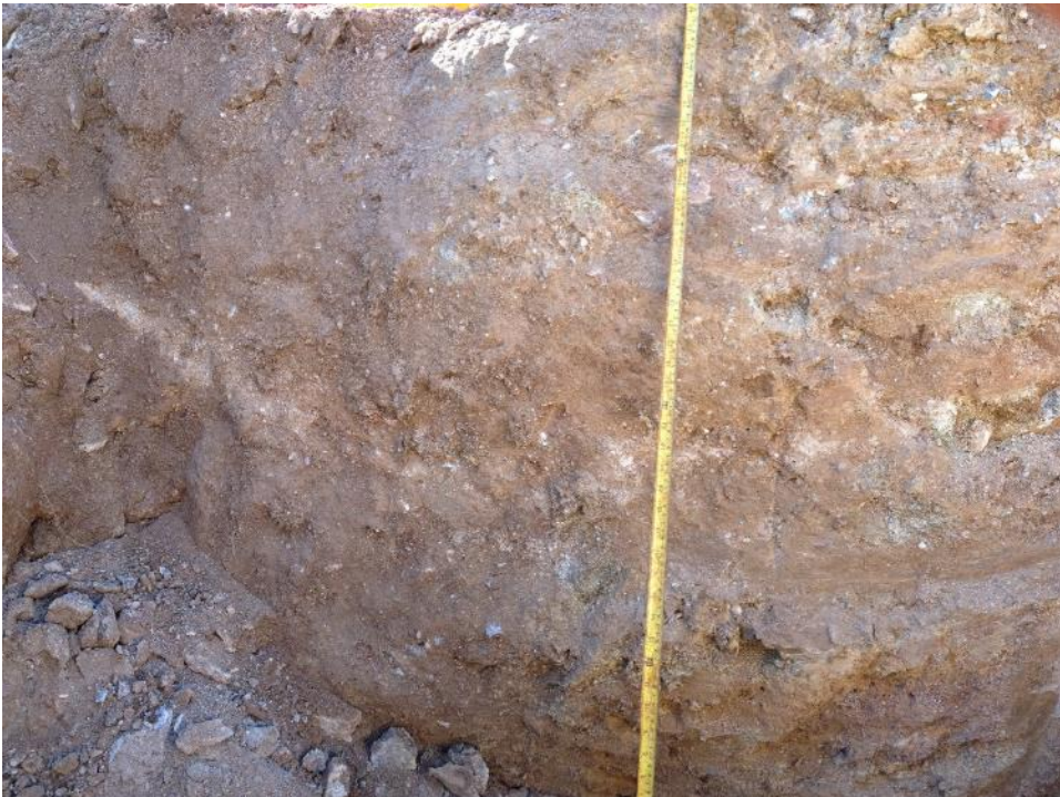
Photo II-20 TP17-35 - 0.8 ft of residual soil overlying slightly weathered Gila Conglomerate. (Mar. 1, 2017)
