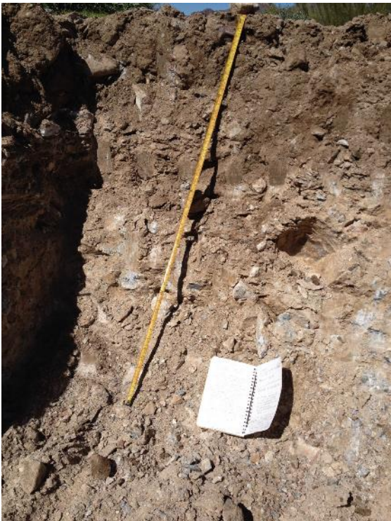
Photo II-28 TP17-37 - Pit excavated in Gila Conglomerate, with 1 foot of residual soil slightly weathered Gila Conglomerate. (Mar. 1, 2017)
