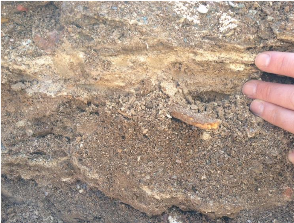
Photo II-15 TP17-34 - Carbonate layer with plant root at 1 ft depth. (Feb. 28, 2017)
