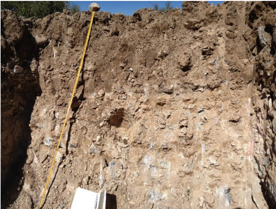
Photo II-29 TP17-37 - Pit excavated in Gila Conglomerate, with 1 foot of residual soil slightly weathered Gila Conglomerate. (Mar. 1, 2017)
