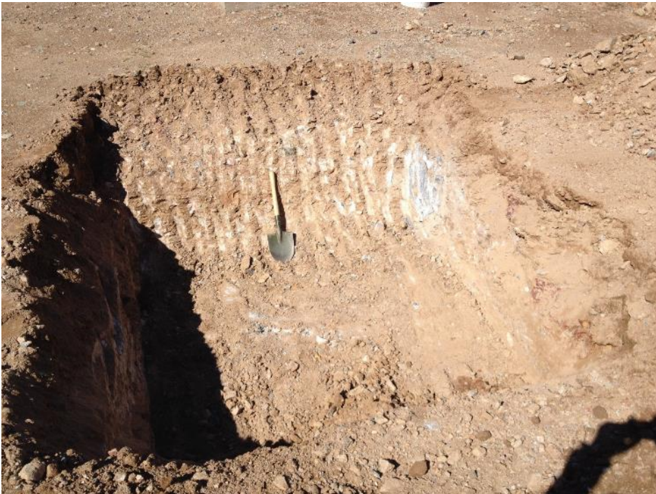
Photo II-24 TP17-36 - Pit excavated in Gila Conglomerate, with 1 foot diameter cobble of schist in right hand corner. (Mar. 1, 2017)
