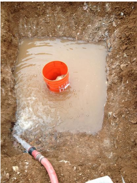
Photo II-8 TP17-32 - Infiltration test in test trench. (Feb. 27, 2017)
