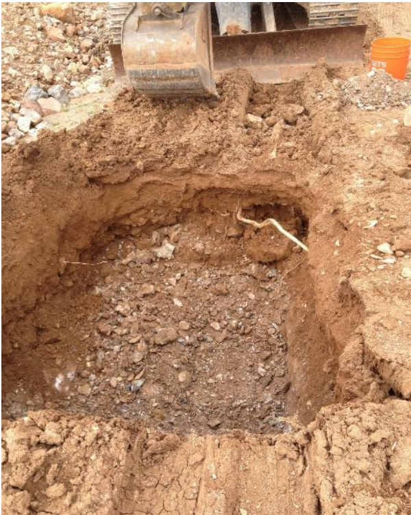
Photo II-5 TP17-32 - 2.5 ft of alluvium composed of gravel, some sand, some silt, overlying Gila Conglomerate in base of trench. (Feb. 27, 2017)
