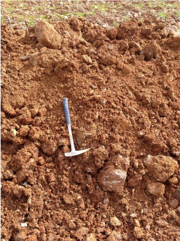
Photo II-3 TP17-31 - Clayey gravel alluvium/colluvium excavated from the trench. (Feb. 27, 2017)
