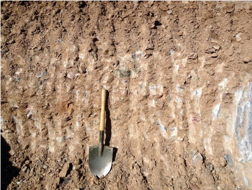
Photo II-25 TP17-36 - Close up of face excavated in Gila Conglomerate. (Mar. 1, 2017)
