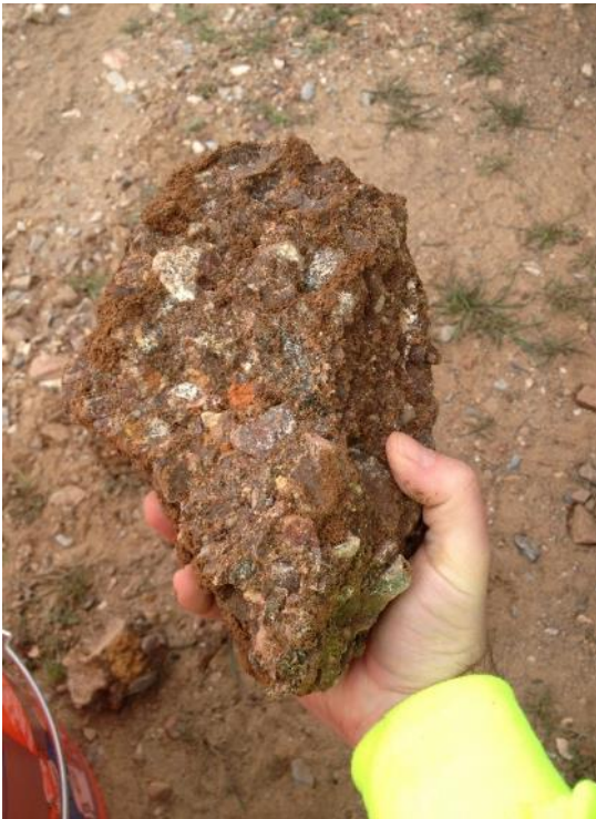
Photo II-7 TP17-32 - Cemented fragment of moderately weathered Gila Conglomerate from 2 ft depth. (Feb. 27, 2017)
