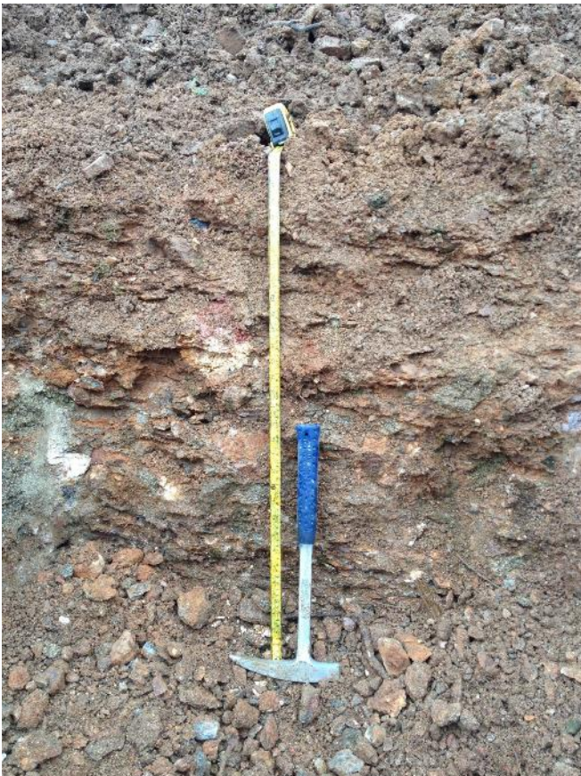
Photo II-10 TP17-33 - 1 ft of compact residual soil overlying highly weathered Gila Conglomerate with rusty mottling. (Feb. 28, 2017)
