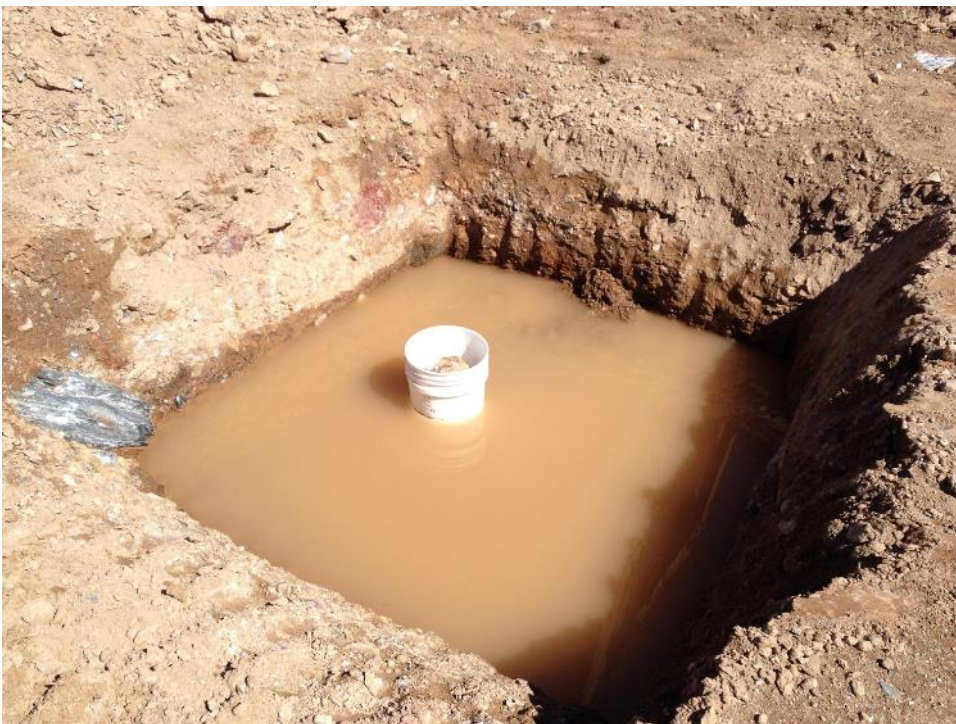
Photo II-26 TP17-36 - Infiltration test in test trench. (Mar. 1, 2017)
