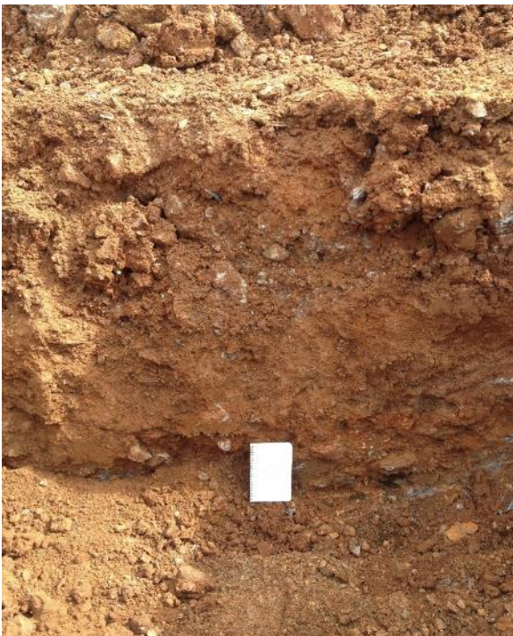
Photo II-2 TP17-31 - Clayey gravel alluvium/colluvium. (Feb. 27, 2017)
