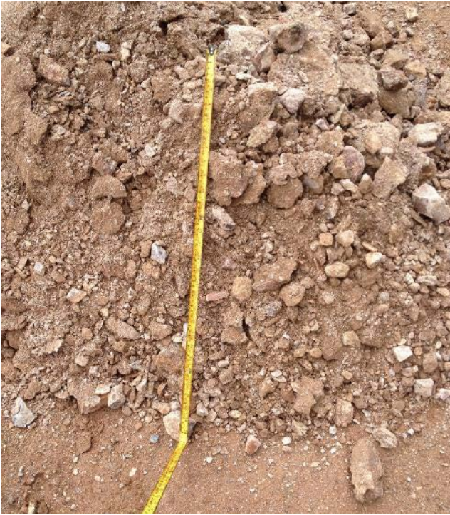
Photo II-17 TP17-34 - Gravel sized fragments of cemented sandstone excavated from trench. (Feb. 28, 2017)
