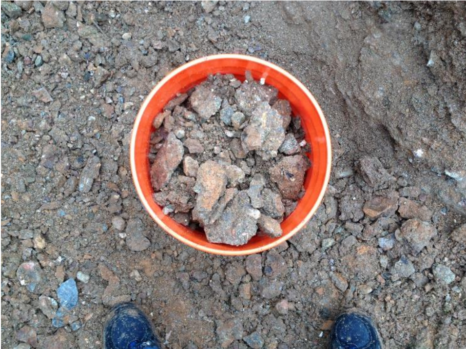
Photo II-11 TP17-33 - Gila Conglomerate excavated from trench, forming gravel size cemented fragments. (Feb. 28, 2017)
