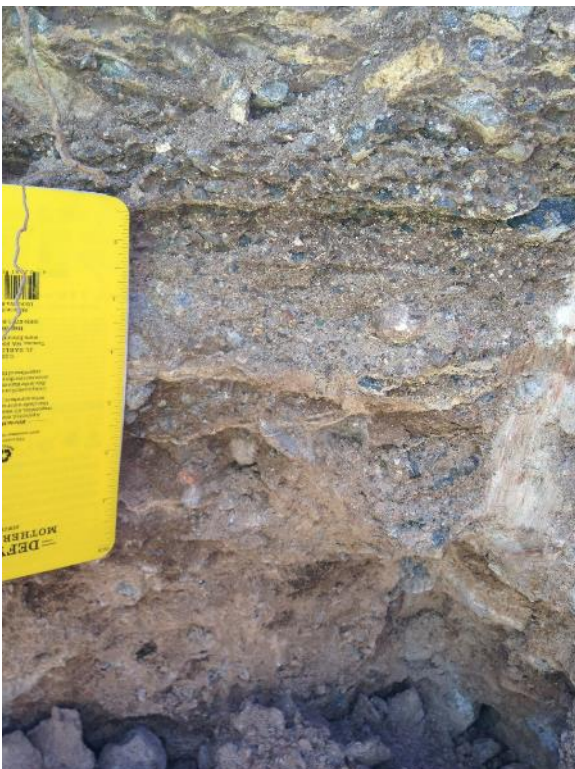
Photo II-30 TP17-37 - Close up of texture of intact Gila Conglomerate. (Mar. 1, 2017)
