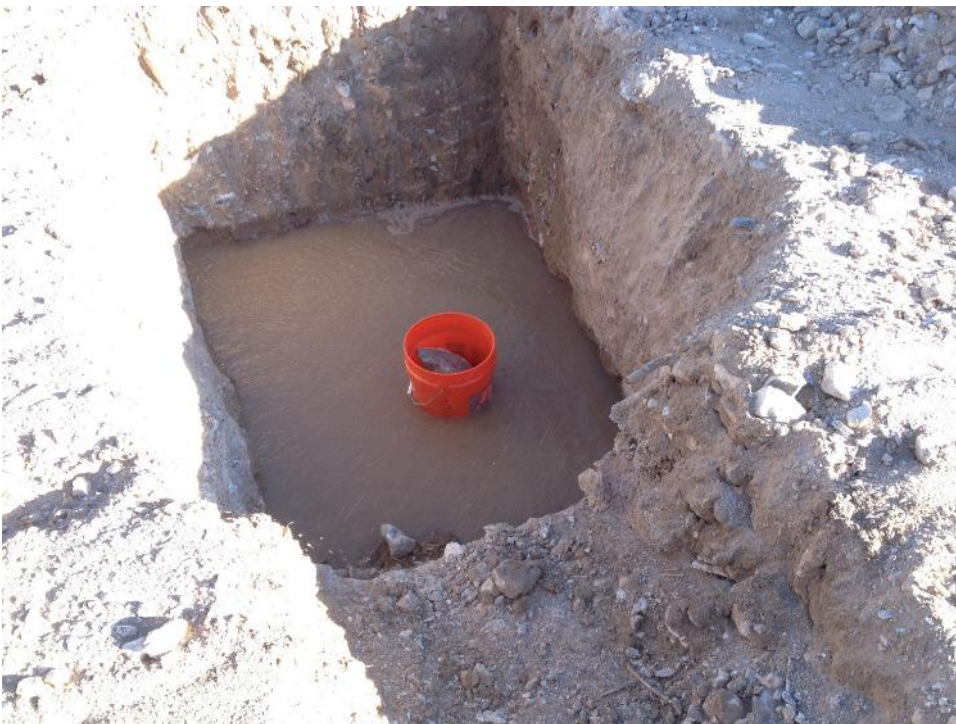
Photo II-32 TP17-37 - Infiltration test in test trench. (Mar. 2, 2017)
