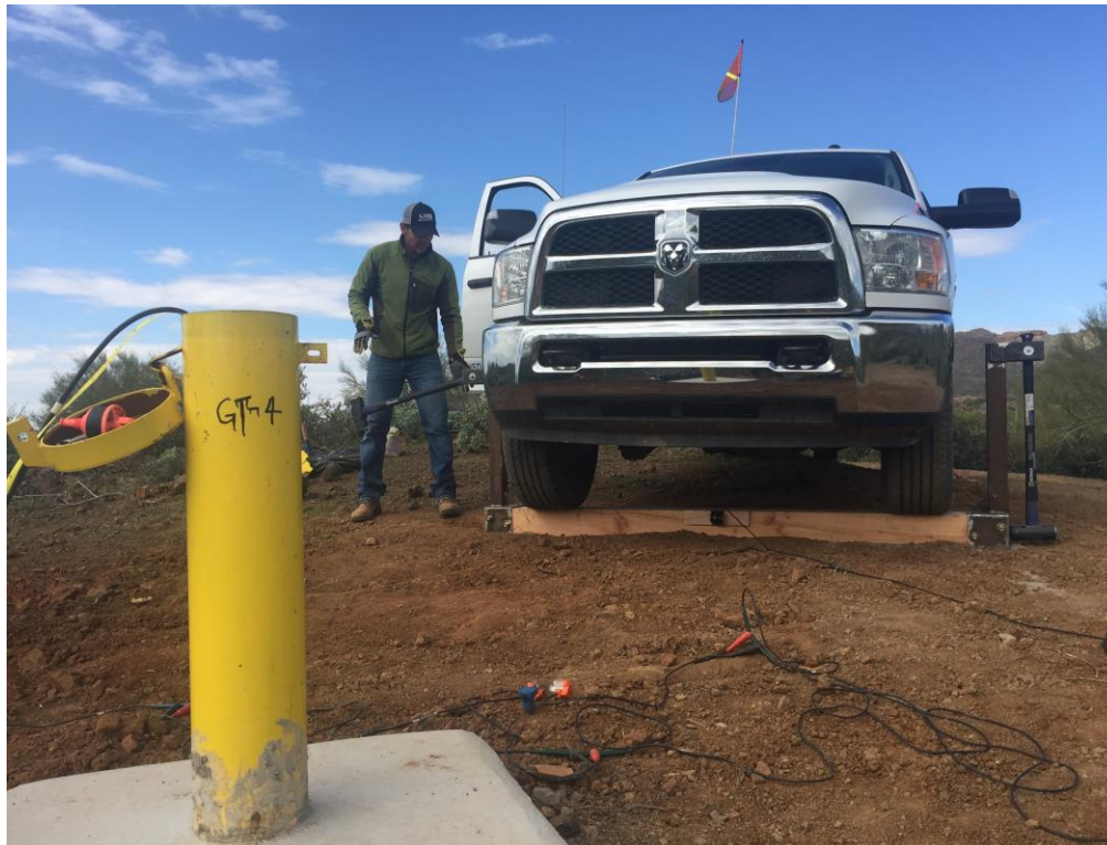
Figure 3. Photograph of the Shear-Wave Pendulum Sledgehammer and Weighted Beam Source System, with the Field Vehicle used to Weight Down the Beam. The Monitoring Geophones for the Shear-Wave Source can be Seen in the Foreground.
