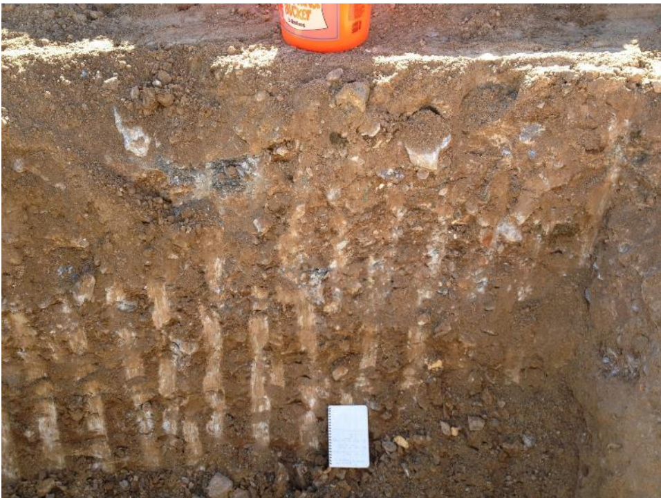
Photo II-34 TP17-38 - Gila Conglomerate exposed in wall of trench. (Mar. 2, 2017)
