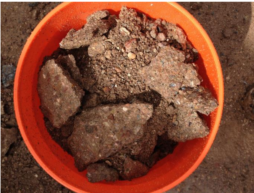
Photo II-18 TP17-34 - Gravel sized fragments of cemented sandstone excavated from trench. (Feb. 28, 2017)
