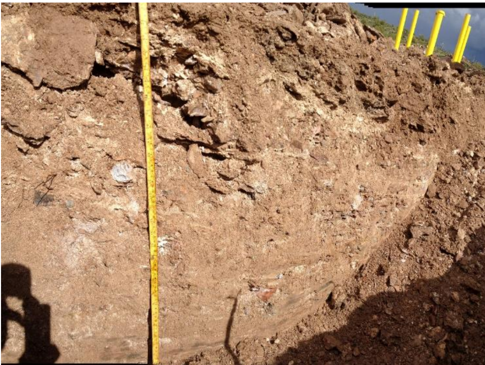
Photo II-16 TP17-34 - Gila Sandstone with 1 ft of highly weathered sandstone with carbonate accumulation along sprung bedding, overlying slightly weathered sandstone. (Feb. 28, 2017)
