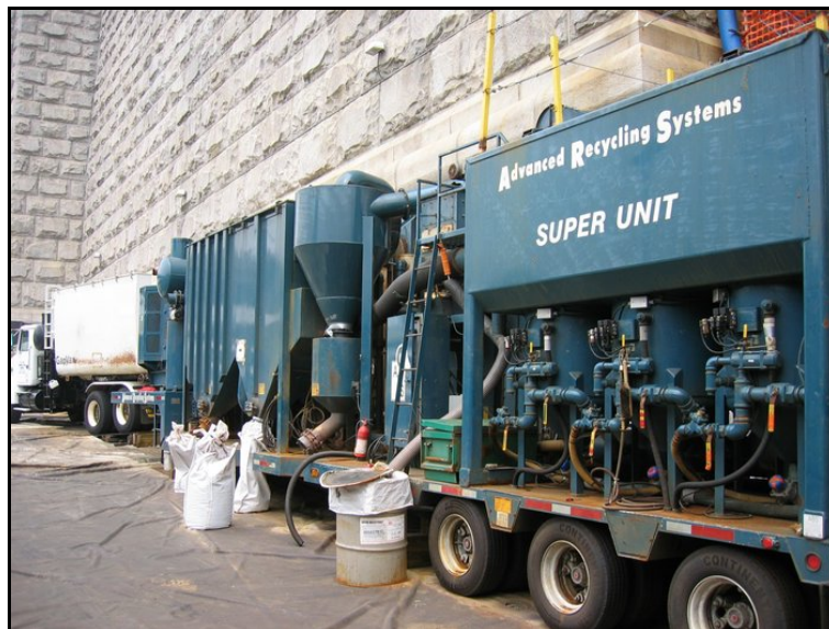
Figure 5.8 Compressors, vacuums, and paint chip collection equipment associated with paint removal operation (Photo #398)
