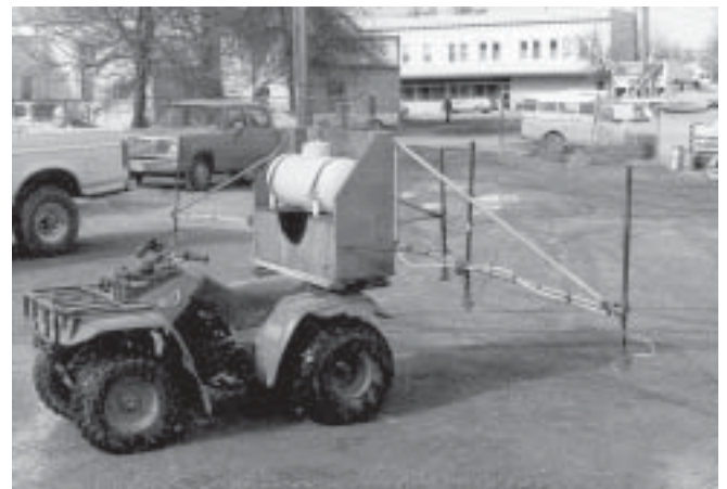
Figure 38 —Boom sprayer mounted on an all-terrain vehicle.
