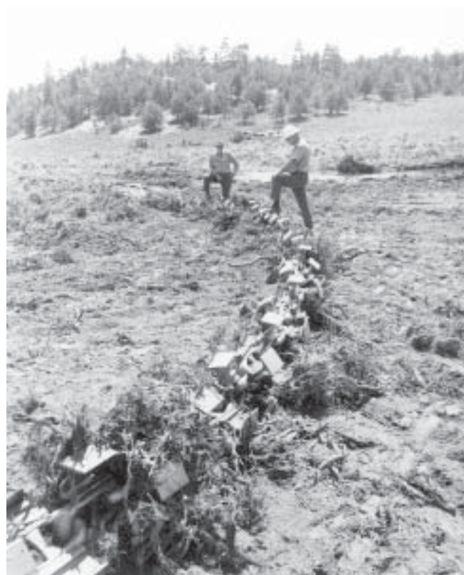
Figure 7—Dixie Sager. Anchor chain with railroad rails welded horizontally to both sides of each link.
