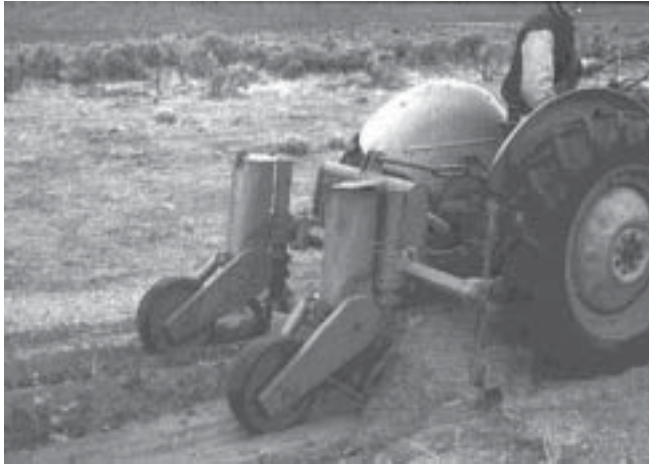
Figure 31 —Two shrub interseeders connected to single tool bar.
