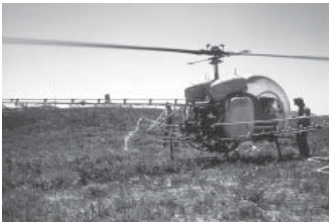
Figure 40 —Helicopter equipped with a boom sprayer.
