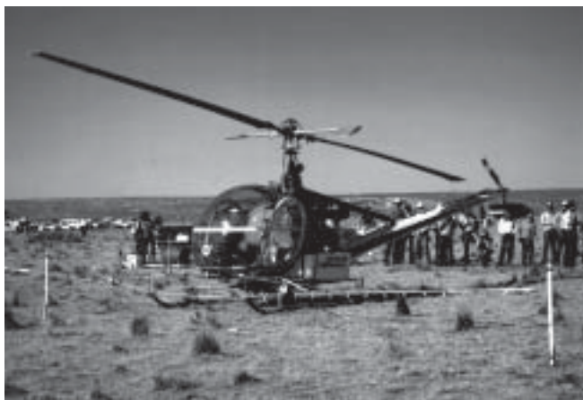
Figure 3 —Helicopter equipped with boom sprayer.
