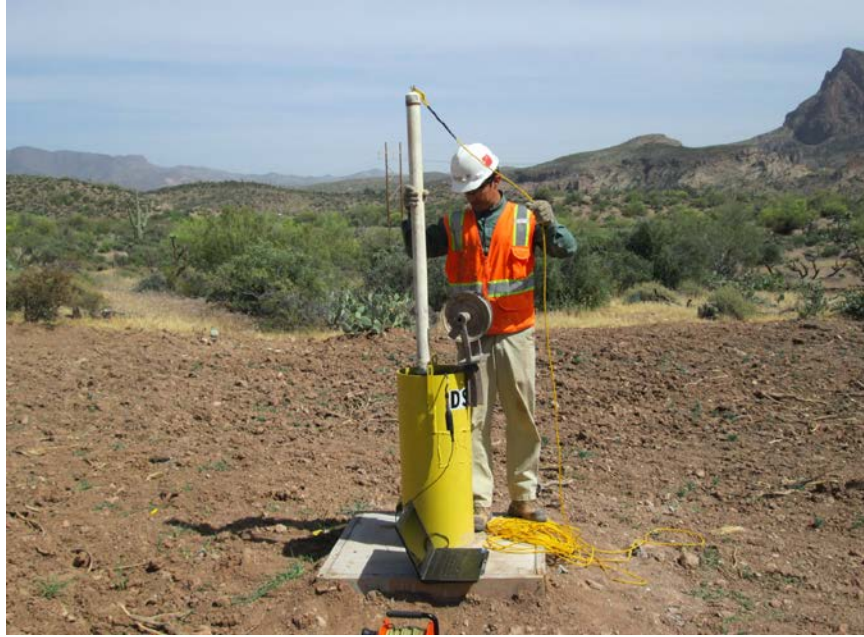
Preparing to conduct falling head slug test at DS17-16
