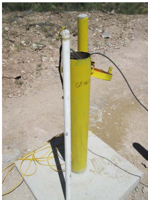
PVC slug next to piezometer DH17-36 (formerly GT-14-3)
