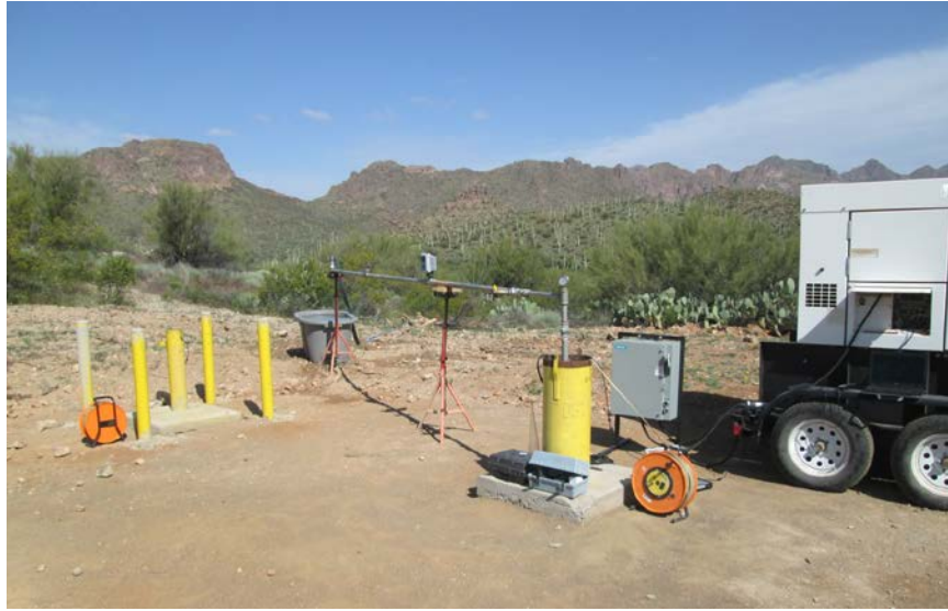
Pumping test discharge assembly and equipment at DS16-07
