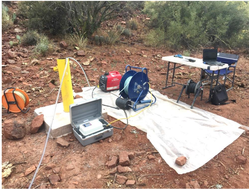
Pumping equipment for short-duration test at DH16-21
