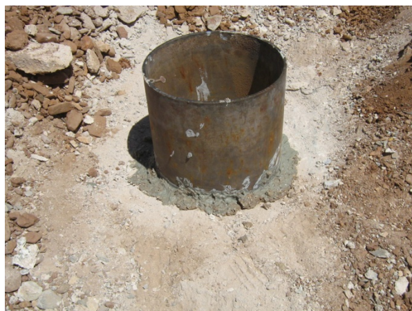
Single-ring (0.30-meter diameter ring), falling-head infiltration test conducted in Test Pit 28 (0.61-meter depth) on strongly cemented caliche surface; hydrated bentonite was used to seal edges of ring in shallow groove on test surface.
