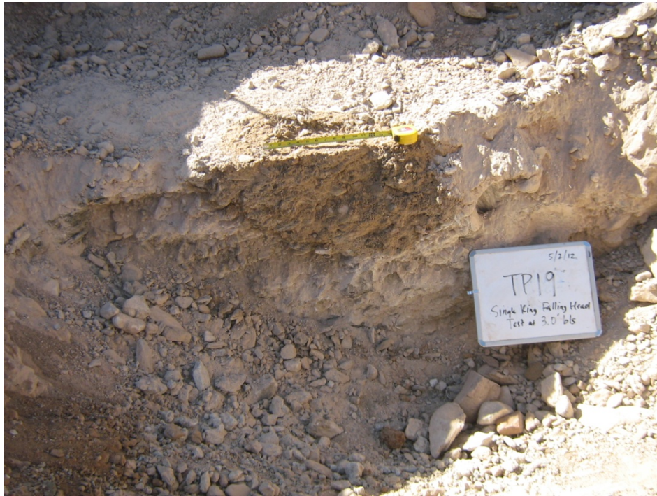
Cross-sectional wetting pattern below surface of single-ring falling-head test conducted in Test Pit 19 (0.91-meter depth) on strongly-cemented caliche surface (tape measure indicates width of ring footprint); significant vertical infiltration occurred with some lateral flow.
