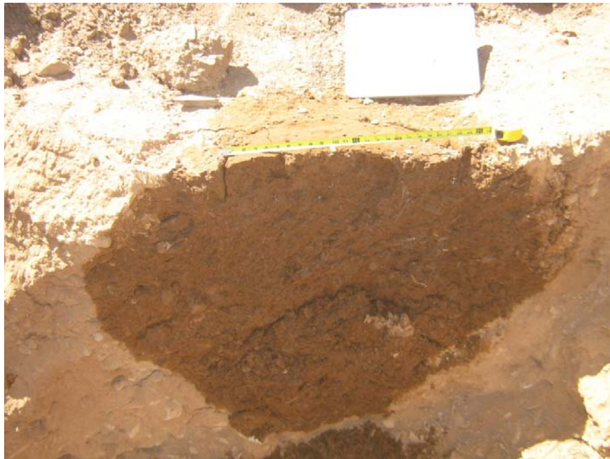
Cross-sectional wetting pattern below surface of double-ring test conducted in Test Pit 24 (0.46-meter depth). Test was conducted in unconsolidated, poorly-sorted sediments and exhibited substantial lateral flow (even in the absence of an underlying caliche layer) due to small-scale heterogeneities.
