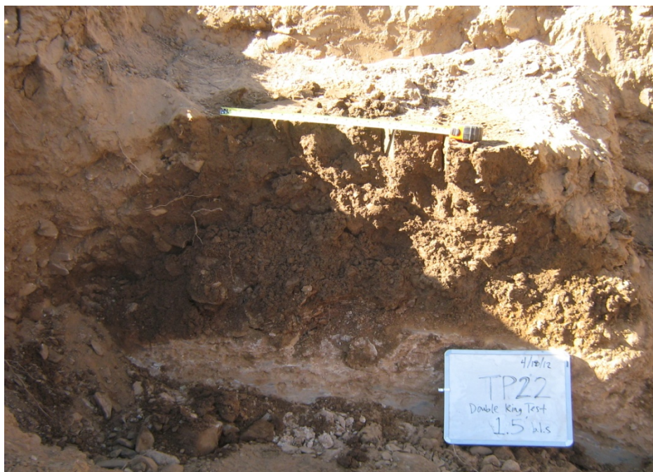
Cross-sectional wetting pattern below surface of double-ring test conducted in Test Pit 22 (0.46-meter depth); the wetting pattern indicates substantial lateral flow above the underlying caliche contact, with little infiltration into it.
