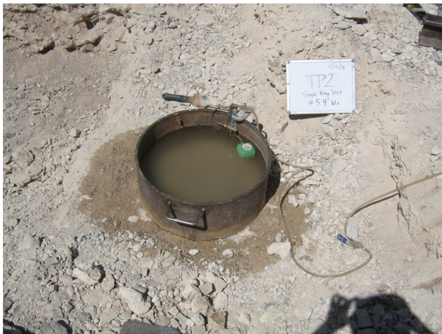
Single-ring infiltrometer (0.61-meter diameter ring) test conducted in Test Pit 2 (1.65-meter depth) in moderately to weakly cemented caliche; the ring was able to be driven into the caliche surface.
