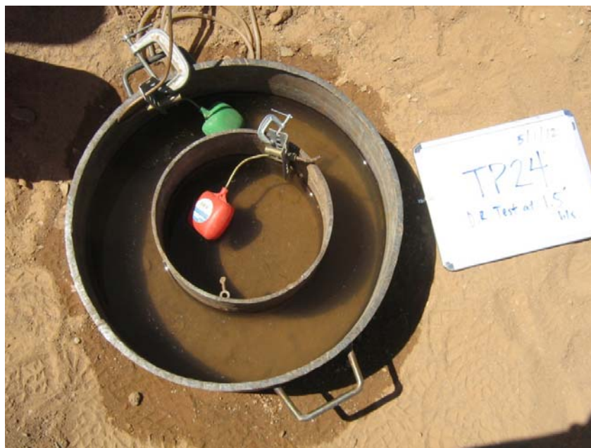
Double ring-infiltrator with float valves to maintain constant hydraulic head during the test.
