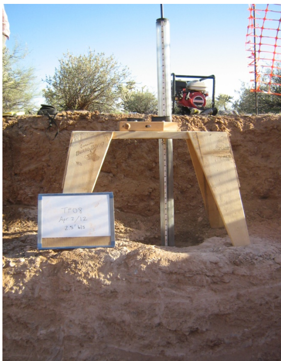
Constant-head permeameter test conducted in strongly-cemented caliche at Test Pit 8 (0.76-meter depth).
