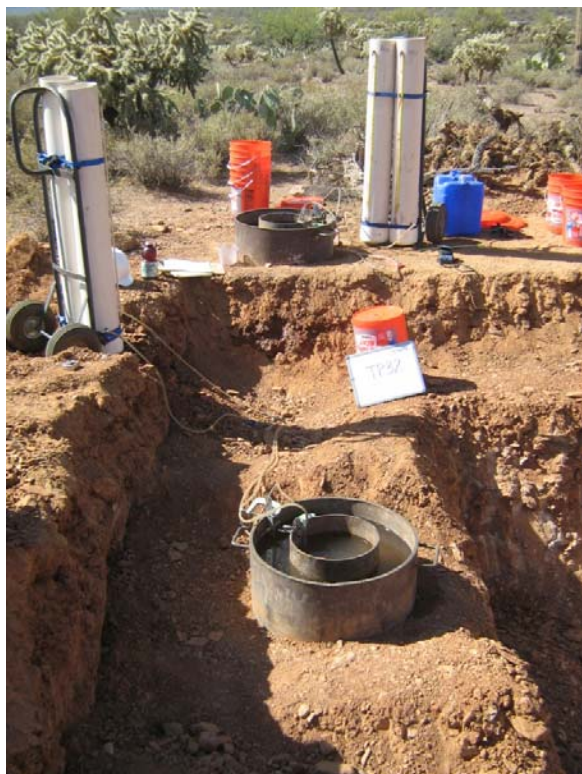
Double-ring infiltrometer tests conducted in Test Pit 32 (left photo) and Test Pit 8 (right photo) on shallow benches.
