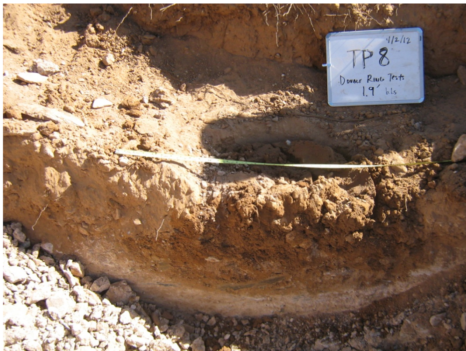
Cross-sectional wetting pattern below surface of double-ring test conducted in Test Pit 8 (0.58-meter depth); the wetting pattern indicates notable lateral flow above the underlying caliche contact, with little infiltration into it.
