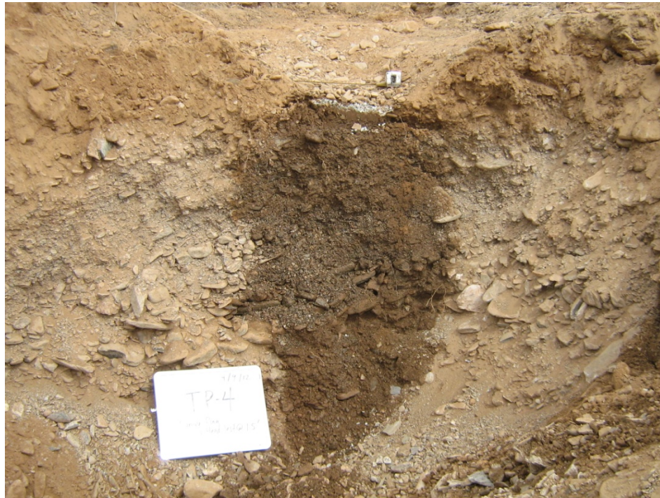
Cross-sectional wetting pattern below surface of single-ring falling-head test conducted in Test Pit 4 (0.46-meter depth) in very gravelly unconsolidated sediments (channel deposits); infiltration was very rapid and chiefly vertical.
