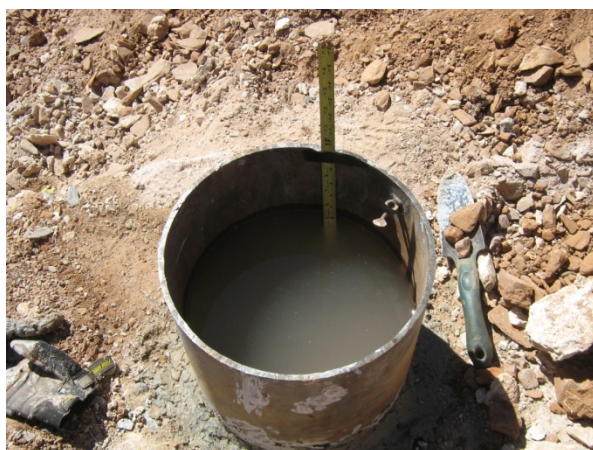
Single-ring (0.30-meter diameter ring), falling-head infiltration test conducted in Test Pit 28 (0.61-meter depth) on strongly cemented caliche surface; hydrated bentonite was used to seal edges of ring in shallow groove on test surface.
