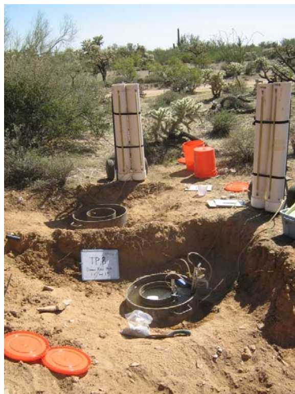
Double-ring infiltrometer tests conducted in Test Pit 32 (left photo) and Test Pit 8 (right photo) on shallow benches.
