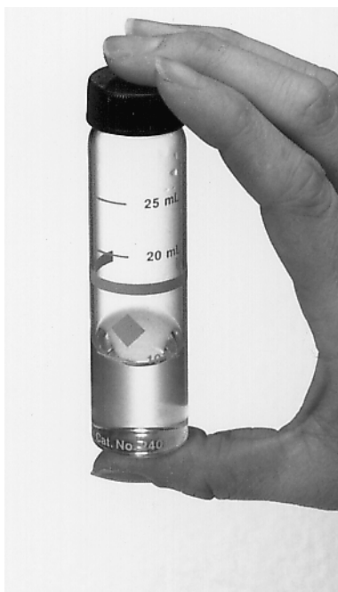
Figure 5 Swirling a Graduated Cylinder
