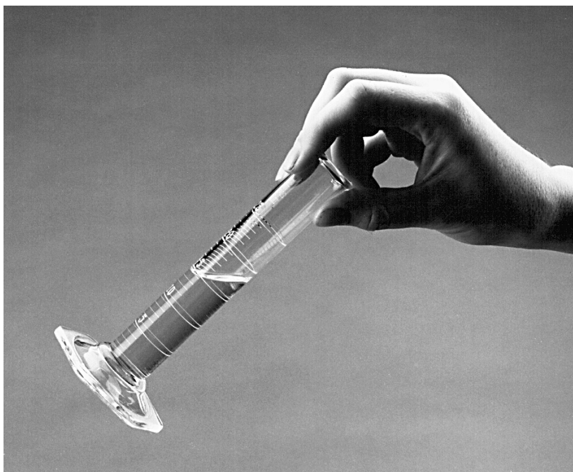
Figure 5 Swirling a Graduated Cylinder
