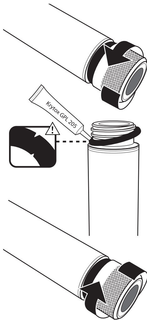
Figure 66 ProDSS ODO cap replacement
