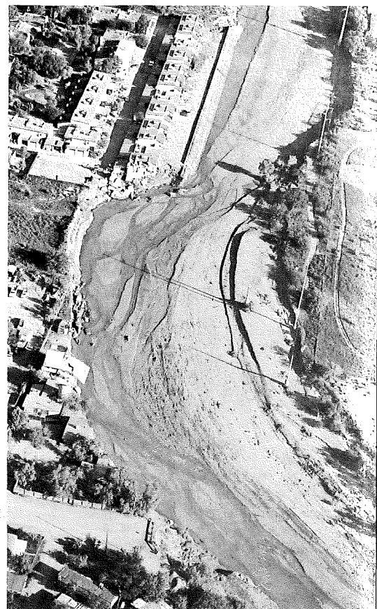
Figure 8. Bank-cutting at outside of bend along west bank of Pantano Wash, south of Golf Links Road. Photo taken on October 9, 1983 by Peter Kresan.
