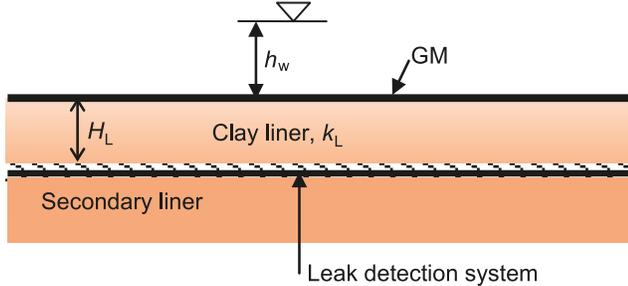
**Fig. 7.** Single composite liner over an attenuation layer and aquifer (also depicts secondary composite liner in a double lined system).
