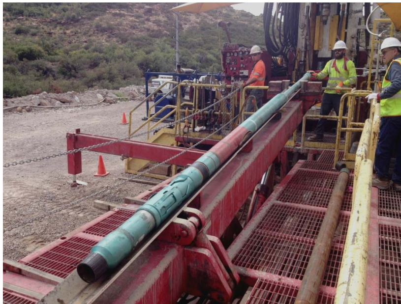
TIW Casing Hanger at DHRES-15
