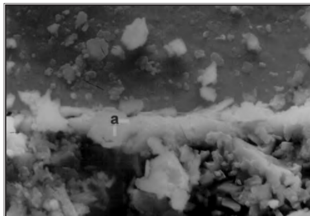
▲ FIGURE 20.9 —SEM photomicrograph of a pyrite grain (top half of photo) and primary hydrothermal-alteration rind (bottom half) in waste-rock piece no. 1. The small platy particles on the pyrite are aluminosilicates, based on EDX spectral analyses. Point a referenced on Figure 20.12.
