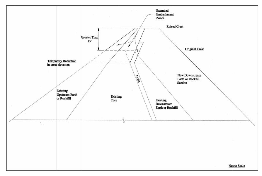
Figure F-8. Downstream raising of embankment dam
