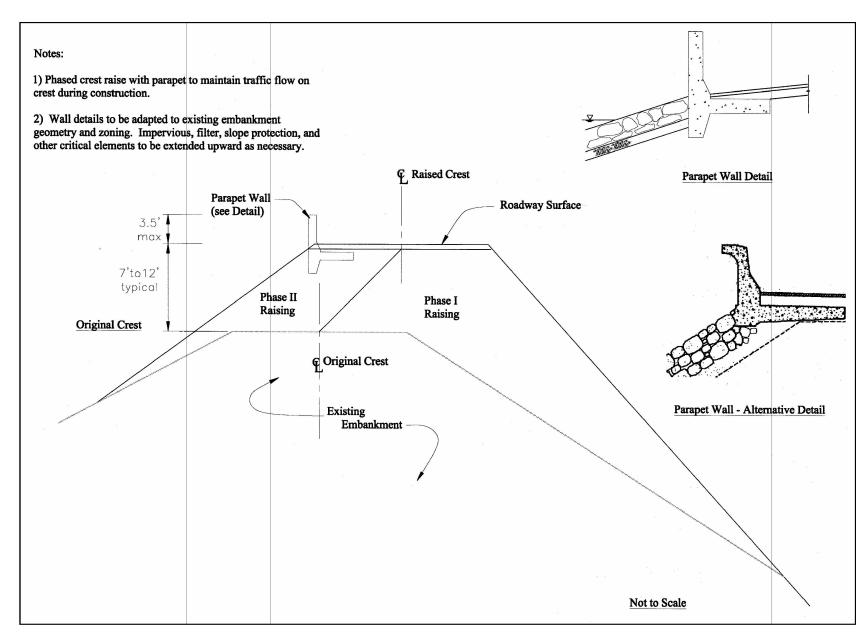
Figure F-4. Embankment raising with parapet wall
