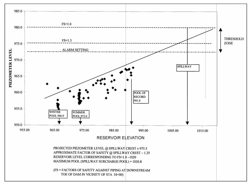
Figure E-3. Load – response (piezometer level versus reservoir elevation) at toe of dam at approximately sta 34+00
