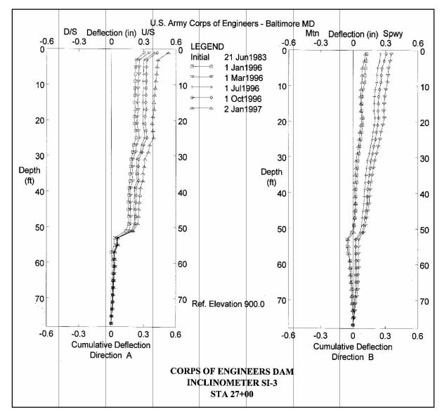
Figure E-5. Typical inclinometer plot
