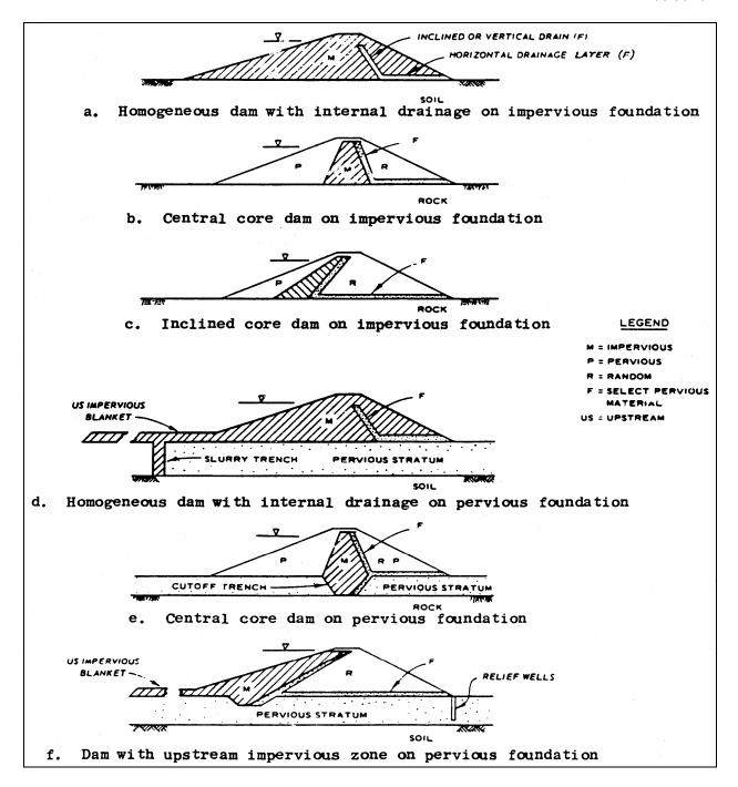
Figure 2-1. Types of earth dam sections
