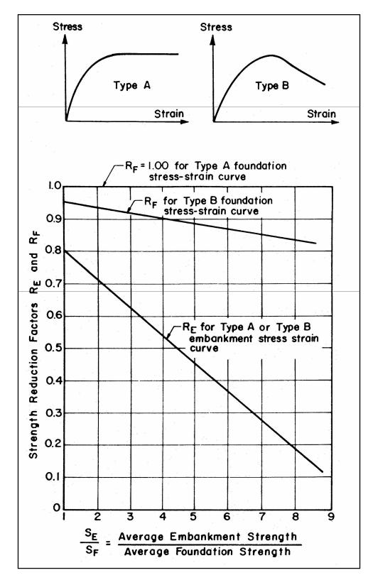
Figure 7-5. Peak strength correction factors for both embankment and foundation to prevent progressive failure in the foundation for embankments on soft clay foundations (Duncan and Buchignani 1975)
