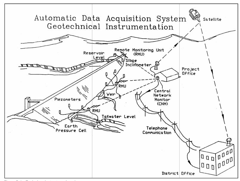
Figure D-1. Typical project automation plan
