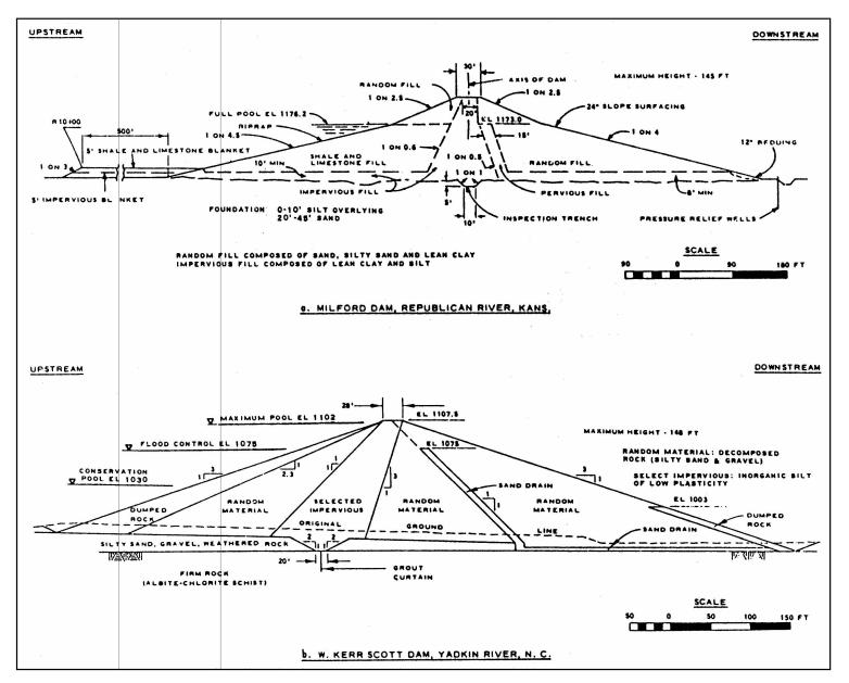
Figure 7-2. Typical embankment sections, earth dams (Milford and W. Kerr Scott Dams)
