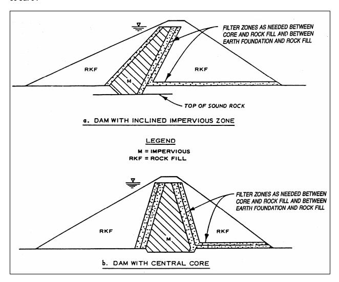
Figure 2-2. Two types of rock-fill dams
