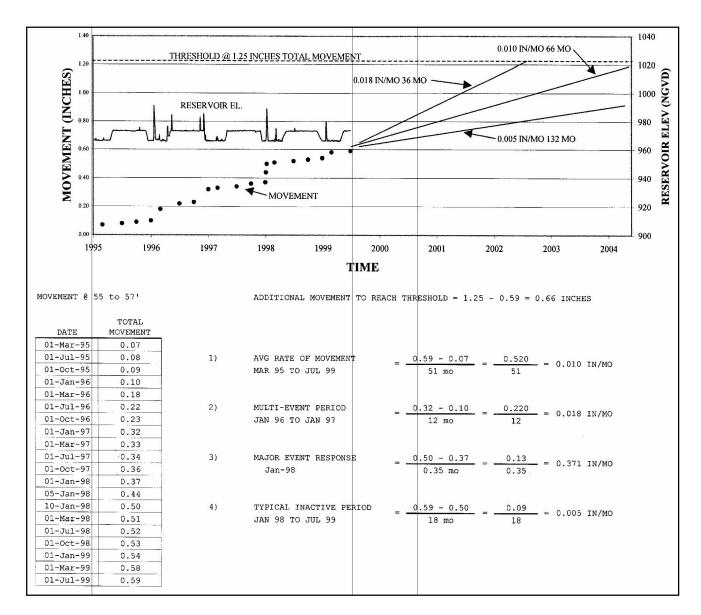
Figure E-4. Deflection/threshold movement
