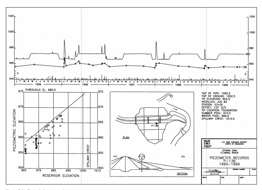
Figure E-2. Typical piezometer plot
