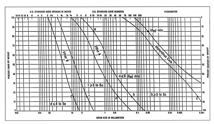
Figure B-2. Illustration of the design of a graded filter
