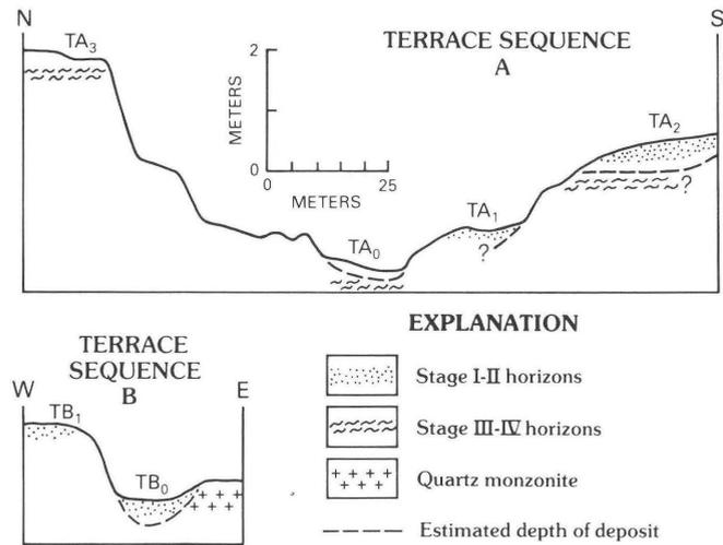
Figure 19. Cross sections of terrace sequences A and B in Gold Valley.
