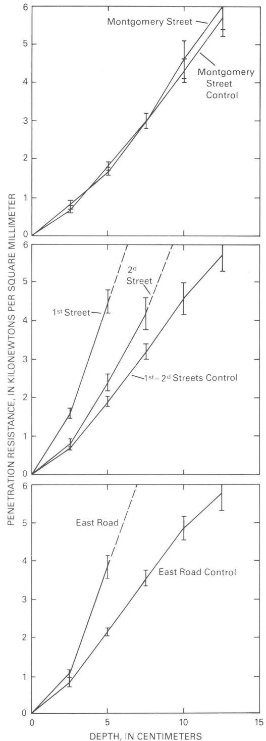
**Figure 15.** Penetration resistance vs. depth curves for soils at Skidoo townsite. Bars indicate standard error, and dashed lines indicate that the next measurement is off-scale.
