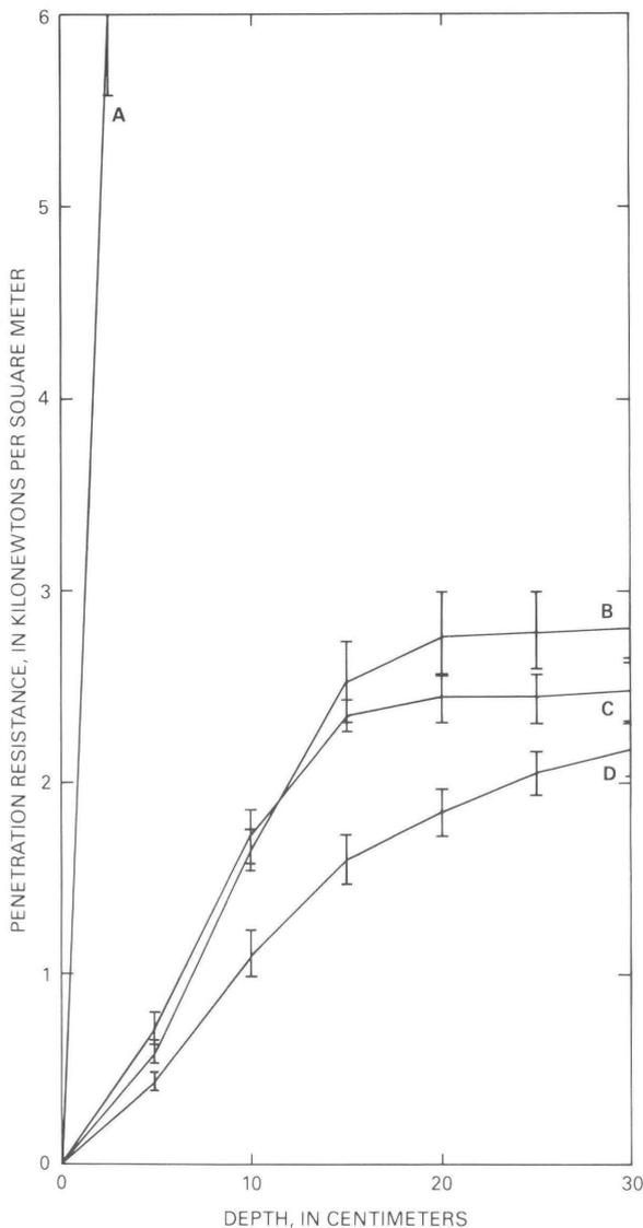
Figure 22. Penetration resistance vs. depth curves for soils at Gold Valley townsite. A, active road; B, western townsite; C, eastern townsite; D, terrace TC<sub>3</sub> control. Bars indicate standard error.
