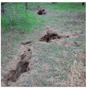
**Photo 47.** Holes in ground, suspected to have resulted from subsidence; no evidence of buried debris was visible.
