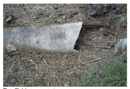
Photo 28. Asbestos concrete pipe.
