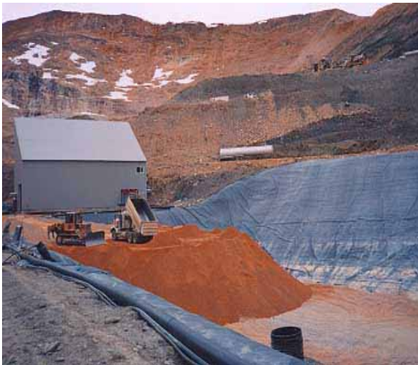
Figure 47: Gold heap leaching
