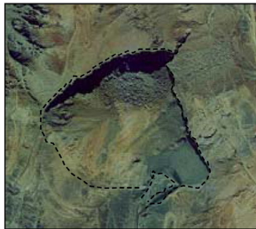
Photograph 9.9: Typical subsidence crater of a block caving mine, II Panel, Andina Mine, Chile.
