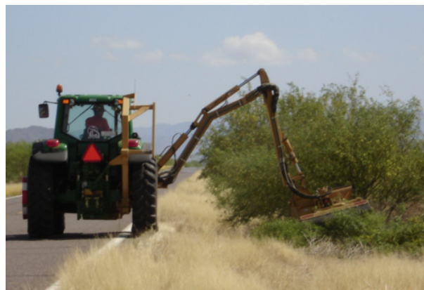
Figure 11.5 A boom axe used to remove trees and brush.
