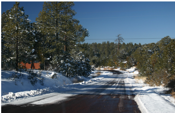
Figure 11.4 Shading on pavement in the winter results in icy conditions.
