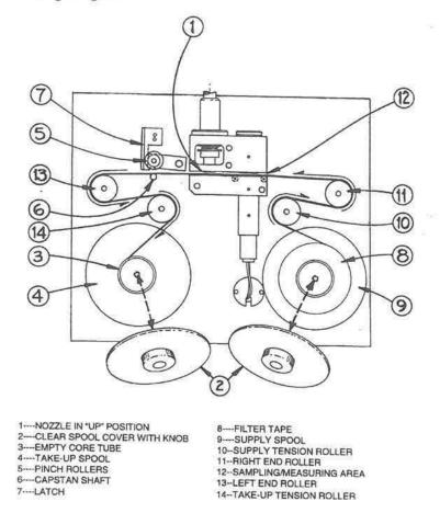
The BAM-1020 has a built-in self-test function that automatically tests most of the tape control and flow systems of the unit. The self-test should be run right after each time the filter tape is changed and can also be used if the operator suspects a problem with the unit. More detailed diagnostic menus are also available for the BAM. They are described in the troubleshooting section of the Operating Manual.
