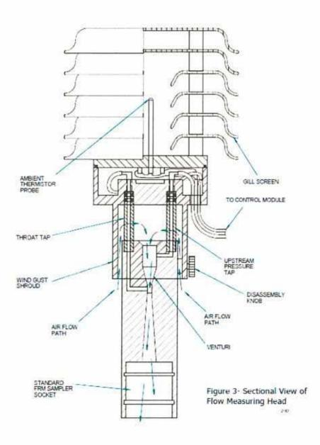
Sectional View of Flow Measuring Head
