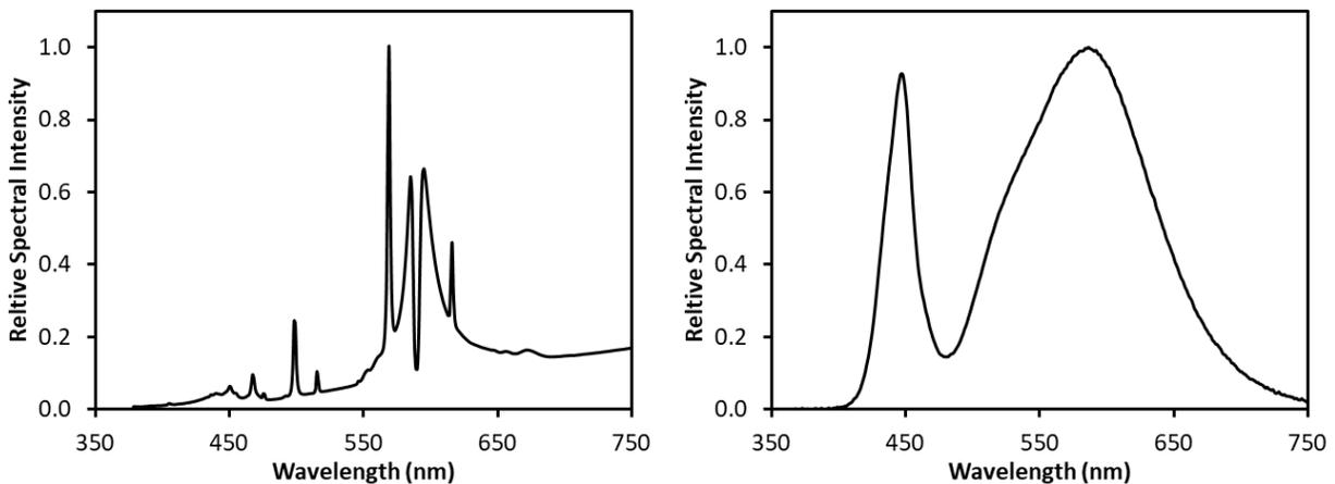
**Figure 10. Relative spectral intensity for the mixed-source HPS/LED/incandescent outdoor lighting spectrum as described in the text (left), and a white LED of 4000K CCT.**
