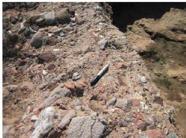
Test **BB-1** (left photo) was conducted on a smoother surface of fine-grained matrix with few small clasts. Test **BB-2** (right photo) was conducted on a rougher surface with many larger clasts cemented in a fine-grained matrix.
