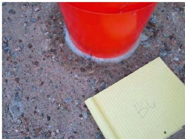
The bucket at test **BB-6** (left photo) was sealed to the test surface exclusively with silicone gel; the test was conducted for 7 hours. Post-test observations for test **BB-6** (right photo) revealed lateral capillary flow within the rock matrix, as seen by the faint ring of wetting up to 7 centimeters from the edge of the bucket.
