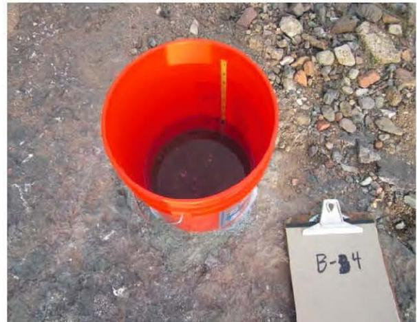
Both silicone gel and bentonite crumbles were used to seal the buckets to the test surface at **BB-3** and **BB-4**, which required some patching after the initial water was added. The tests began after the seal was confirmed to be water tight, and were conducted for 16 hours (including overnight).
