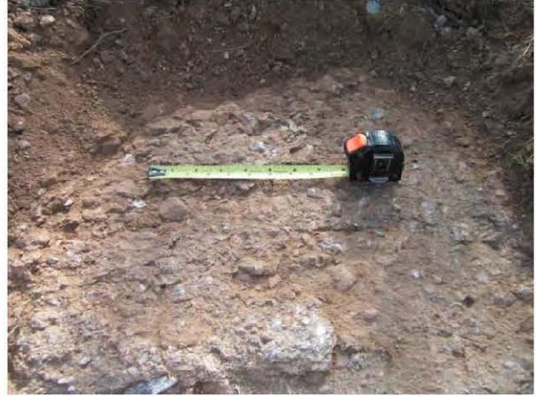
Test **BB-5** (both photos) was conducted in highly weathered/decomposed conglomerate, in which a relatively hard surface was exposed and cleared; the test zone included layers of bedrock and "soil" with subsurface horizontal bedding planes.
