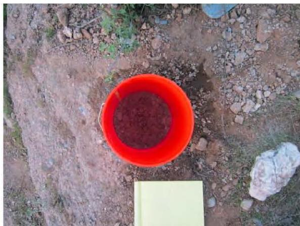
The bucket at test **BB-5** (left photo) was sealed to the test surface exclusively using hydrated bentonite crumbles; the test was conducted for 7 hours. Post-test observations for test **BB-5** (right photo) revealed substantial lateral flow (both saturated and capillary flow) along the subsurface bedding planes and in the "soil" zones.
