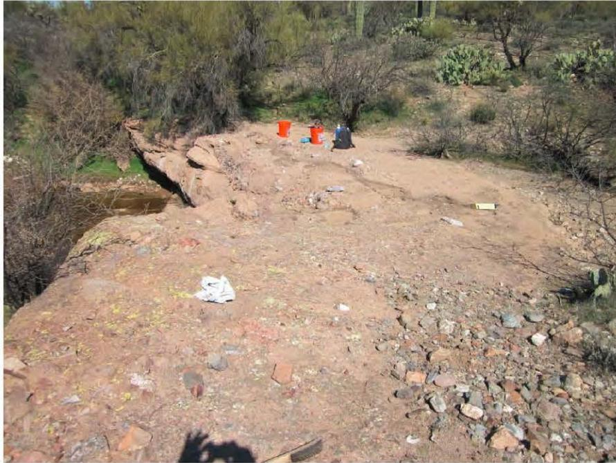
Infiltration tests **BB-1** and **BB-2** were conducted on a bedrock outcrop of Gila Conglomerate (Tcg), located above Benson Spring. The outcrop was characteristic of well-lithified, poorly sorted conglomerate.
