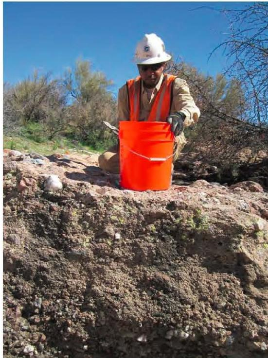
The “Bottomless Bucket” infiltration test method was used to conduct tests on the bedrock surfaces. Quick-drying silicone gel and hydrated bentonite crumbles were used to seal the bucket to the test surface and prevent leakage.
