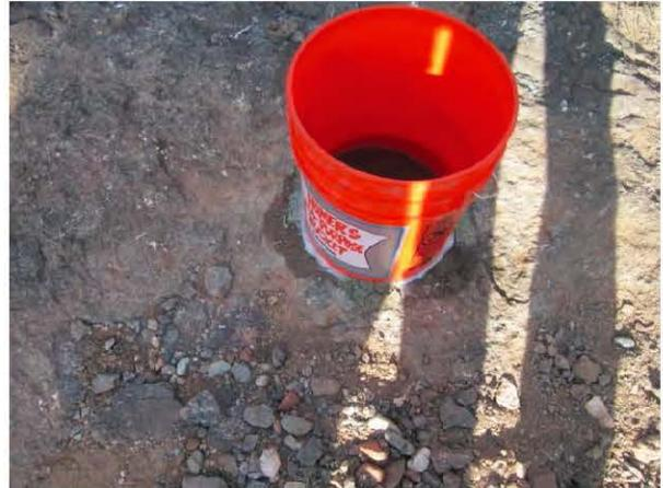
Test **BB-3** (left photo) demonstrated substantial lateral flow through the extensive shallow fractures at the surface. The distance of lateral wetting ranged up to 60 centimeters from the edge of the bucket. Test **BB-4** (right photo) demonstrated a small amount of lateral capillary flow in the rock matrix, as shown by the faint ring of wetting extending about 5 centimeters from the edge of the bucket.
