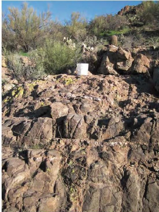
Test **BB-7** was conducted on an outcrop of Apache Leap Tuff vitrophyre (Talv), located in Roblas Canyon.
