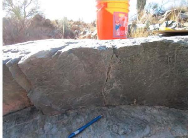
The test surface at **BB-8** was relatively smooth and contained several fine fractures and one fracture with a surface aperture up to 1 centimeter; the vertical extent of selected fractures may have been significant (right photo). Silicone gel was used exclusively to seal the bucket to the test surface.
