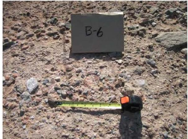
Test **BB-6** (both photos) was conducted on a well-lithified and non-fractured conglomerate surface that included poorly-sorted clasts in a fine-grained matrix.
