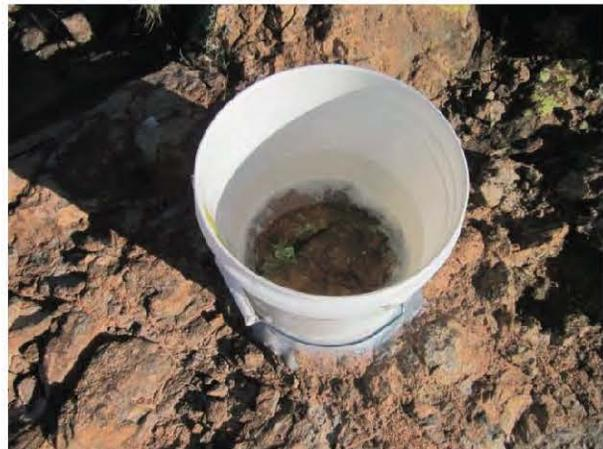
The test surface at **BB-7** was rugged and non-fractured, and the bucket was sealed exclusively with silicone gel.
