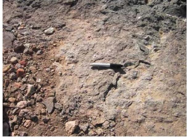
The two basalt surfaces tested at **BB-3** and **BB-4** were distinctly different. Test **BB-3** (left photo) was conducted on a surface with extensive shallow fracturing and quartz/feldspar veining. Test **BB-4** (right photo) was conducted on a relatively smooth and non-fractured surface.
