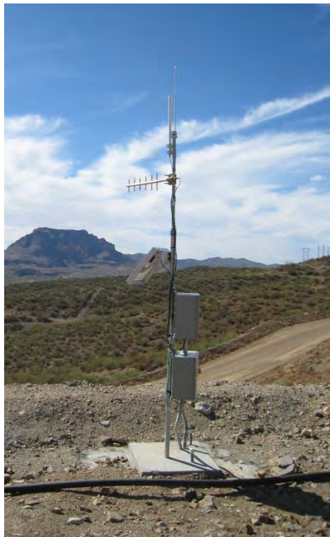
Photograph 6. Telemetry system at DHRES-03/DHRES-04.
