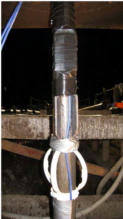
Photograph 4. Transducer strapped within protective fins on 3-inch casing at DHRES-03
