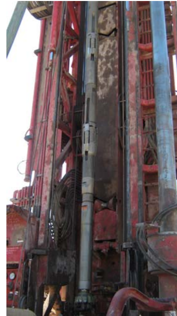
Photograph 3. Air-hammer downhole assembly at HRES-11
