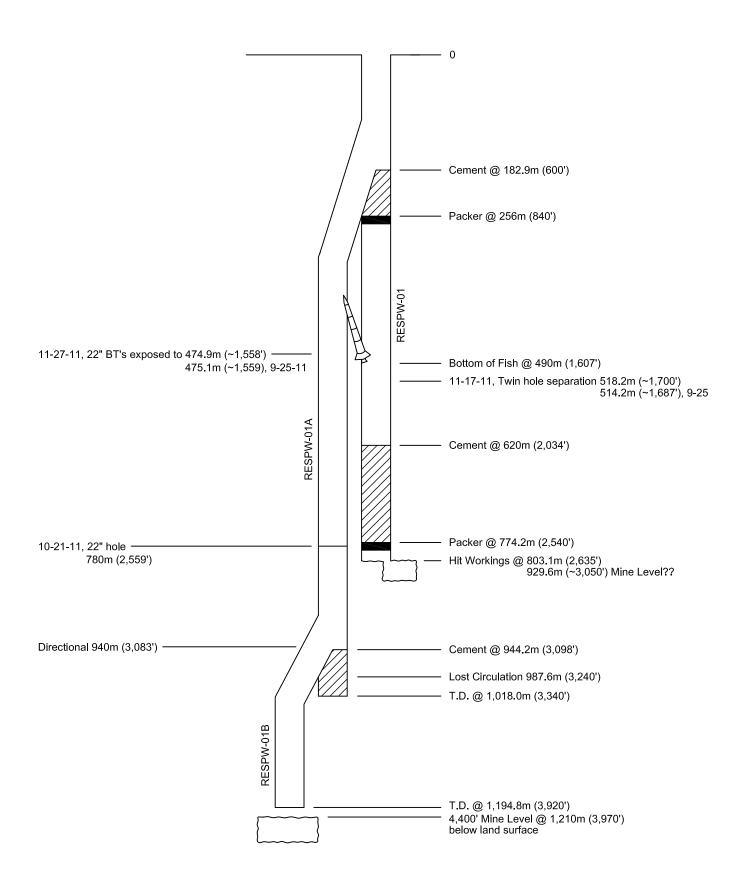
FIGURE 3. SCHEMATIC DIAGRAM OF THREE BOREHOLES AT RESPW-01, RESOLUTION COPPER MINING
