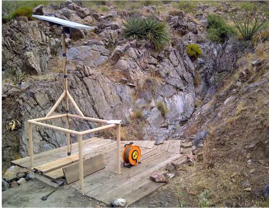
Photo 3. Bitter Spring sump and fracture-controlled canyon upstream, sump collared in quartz diorite, Pinal schist crops out 100 feet upstream, August 2012.
